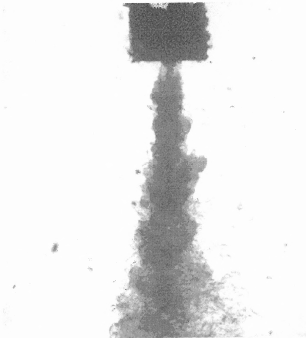
Figure 4.2 Injection of solution into the view cell P = 100 Bar, T = 35 C, V_{sol} = 0.4 ml/min, v = 1.18 m/s, D_{nozzle} = 127 \mu\text{m} , V_{CO_2} = 60 , ( CO_2 pulsations are not induced).
