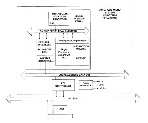
Figure 2.17 Floating-Point Co-Processor.
