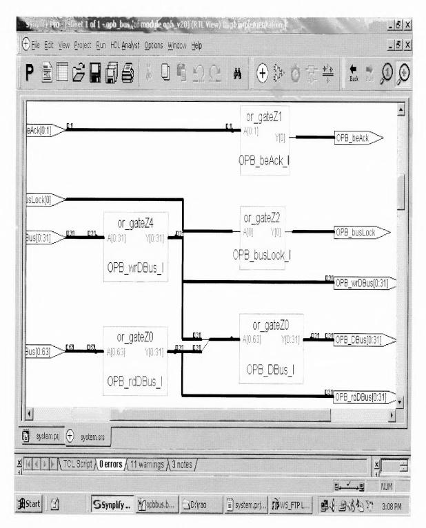
Figure 3.5 Hierarchical view of the OPB bus.
