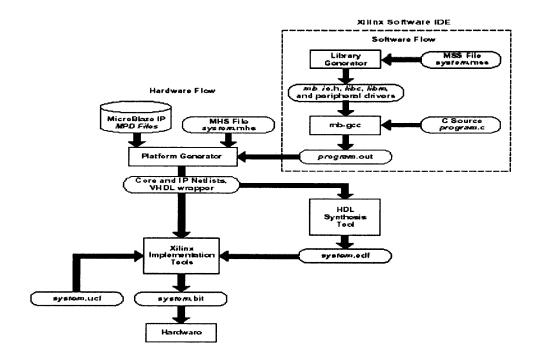
Figure 3.2 Microblaze design flow [13].
