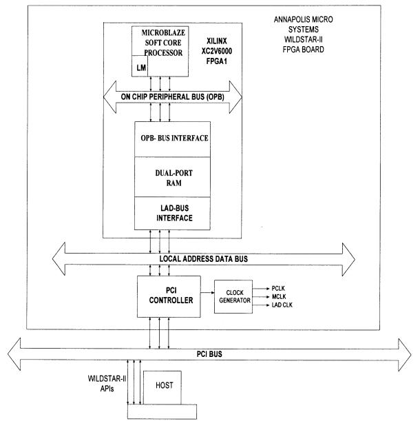
Figure 2.5 Sequential Architecture of Microblaze.
