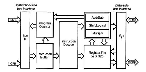
Figure 2.3 Microblaze Core Block Diagram [13].
