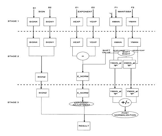
Figure 2.11 3-stage Pipelined Floating-Point Adder/Subtractor.
