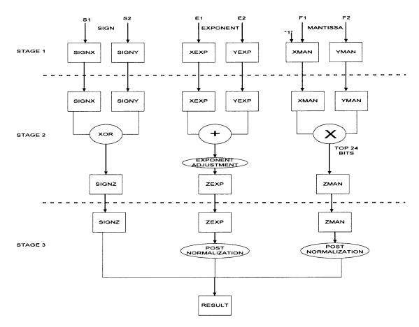
Figure 2.12 3-stage Pipelined Floating-Point Multiplier.
