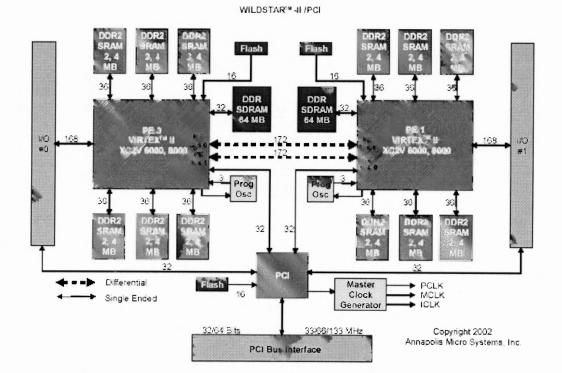
Figure 2.1 Wildstar-II/PCI Block Diagram [14].
