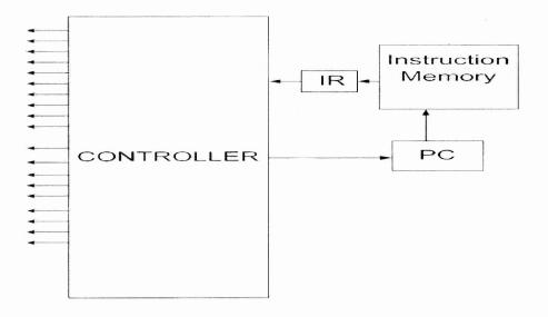
Figure 2.15 Controller of the SIMD machine.
