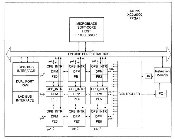
Figure 2.8 Architecture of the SIMD Machine.
