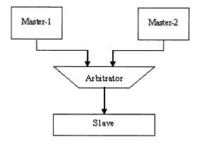
Figure 2.2 Slave-side arbitration in the Avalon bus system.
