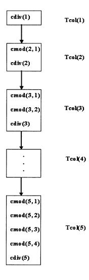
Figure 3.4 Task and subtasks for a matrix of order n = 5.
