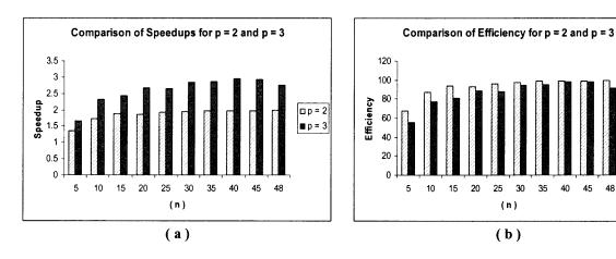
Figure 4.2 Comparison of (a) speedup and (b) efficiency for p = 2 and p = 3.
