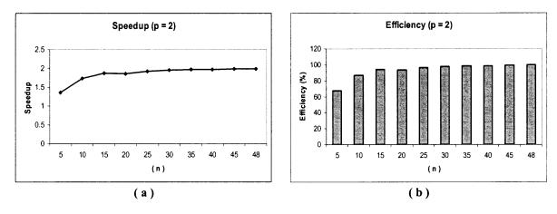
Figure 4.1 (a) Speedup and (b) efficiency for p = 2.
