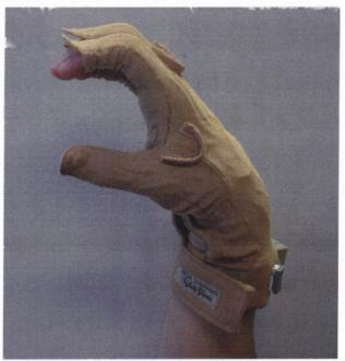
Figure 5.1 A subject with the right Cyberglove on forming the letter C.
