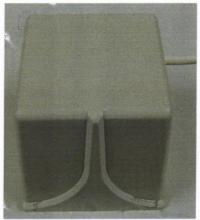
Figure 2.2 The transmitter for the Flock of Birds.
