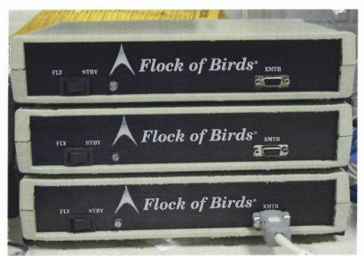
**Figure 2.4** Three Flock of Bird units where each unit contains the transmitter driver and the signal processing electronics are contained.
