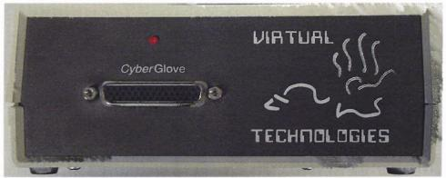
Figure 2.13 The Cyberglove Interface Unit (CGIU).
