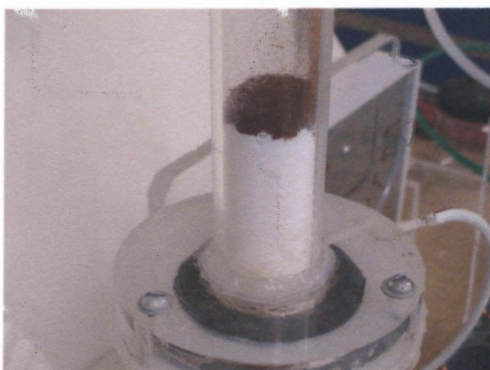
(a) Before fluidization: \text{Al}_2\text{O}_3 (white) and \text{Fe}_2\text{O}_3 (reddish brown)
