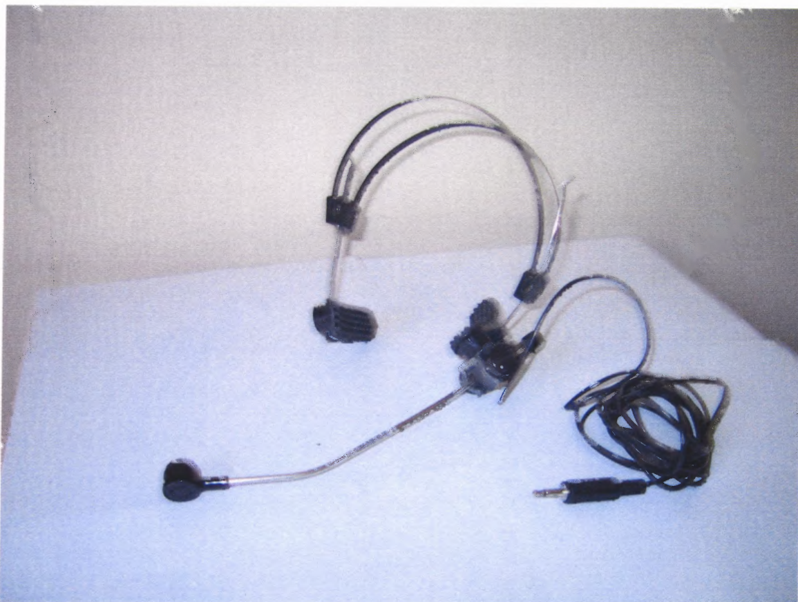
Figure 3.8 Pictured here is the Shure SM10A headset microphone used to capture the audio from the participants' speech. It was connected to the Sony DCR-PC5.
