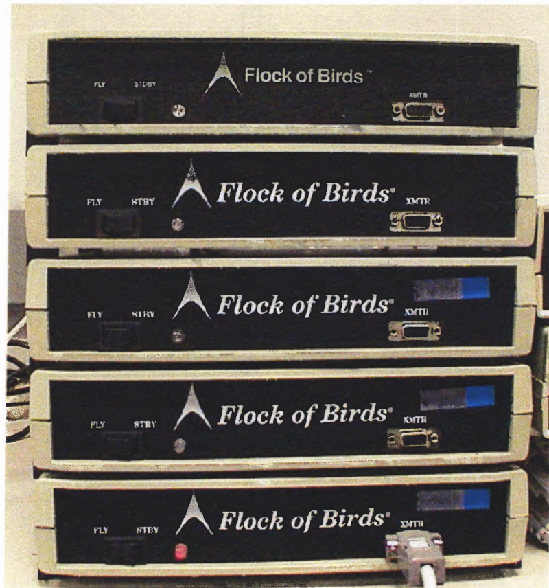
Figure 4.9 The Flock of Bird units where the transmitter driver and the signal processing electronics are contained.
