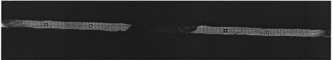
Figure 2.13 AOI location on filament image. Image shows placement of powder coating in the middle of the filament. The four small squares on the filament are the Area of Interest (AOI) selected for processing the filament image for temperature determination.
