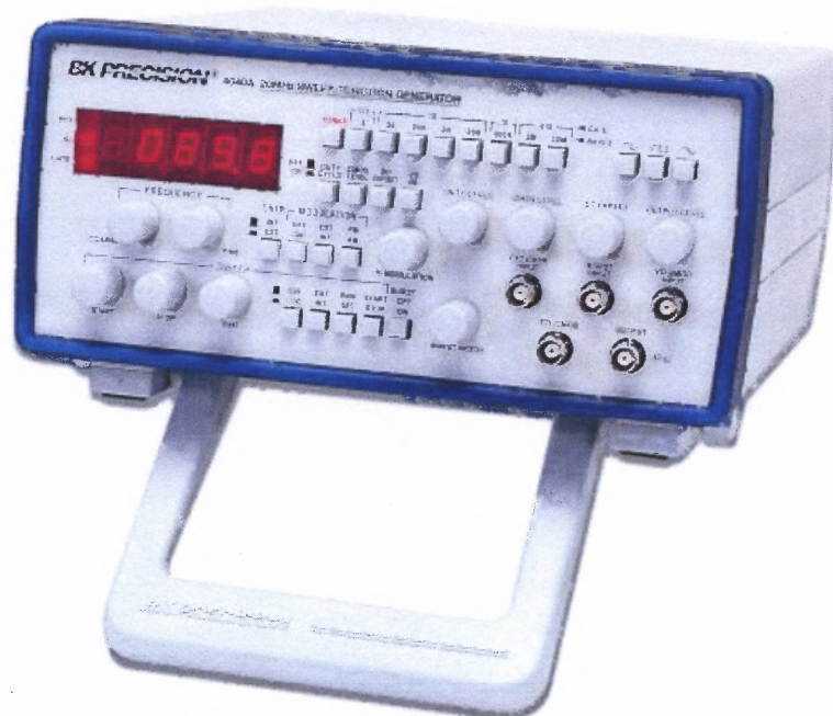
Figure 2.7 BK Precision Model 4040A, 20 MHz Sweep Function Generator [5].
