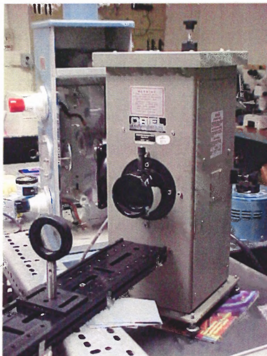
Figure 3.1 Oriel mercury arc lamp with a focusing lens.
