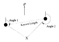
Figure 3.2 Example of 2D angulation illustrates locating object 'X' using angles relative to a  $0^{\circ}$  reference vector and the distance between two reference points. 2D angulation always requires at least two angles and one distance measurement to unambiguously locate an object.
