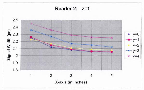
**Figure A.9** Signal width for Reader 2 located at (4,0,4). Tracking tag is on the elevated plane (z = 1). Observations were obtained for five points for each y-axis on the grid of the plane.
