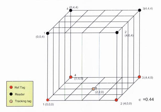
**Figure 4.17** Four tag readers, four reference tags and a tracking tag placed in a  $4" \times 4" \times 4"$  cube. The experimental error rate was found to be 0.44 inches.
