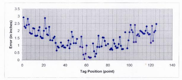
**Figure 4.7** Variation in error rates versus the position of a tracking tag for the configuration as shown in Figure 4.6.
