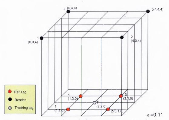
**Figure 4.18** Alternative positions of reference tags, error rate has reduced to  $\in =0.11$  inches.
