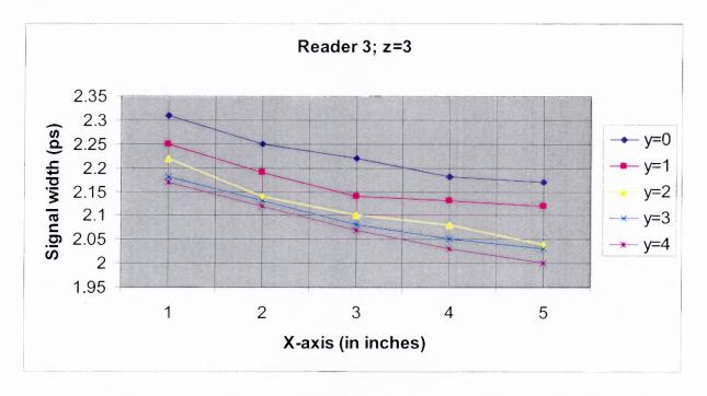
**Figure A.17** Signal width for Reader 3 located at (4,4,4). Tracking tag is on the elevated plane (z = 3). Observations were obtained for five points for each y-axis on the grid of the plane.
