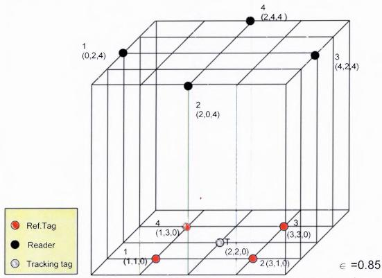
Figure 4.19 Another alternative positions of tag readers caused error rate to increase to  $\in =0.85$  inches.
