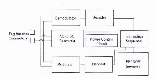
Figure 2.3 Block diagram of a microchip in a passive tag.
