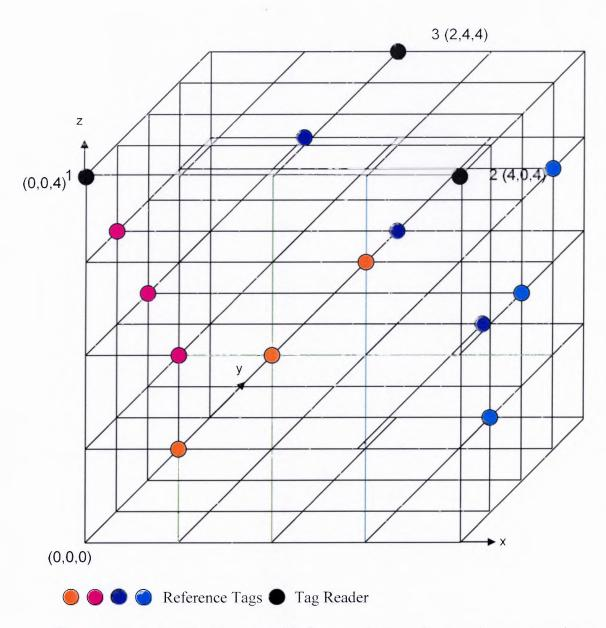
**Figure 4.6** A  $4" \times 4" \times 4"$  cube, with three readers on the top-plane and twelve reference tags diagonally placed on each four vertical planes.
