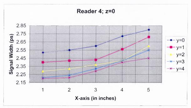
**Figure A.20** Signal width for Reader 4 located at (0,4,4). Tracking tag is on the lowest plane (z = 0). Observations were obtained for five points for each y-axis on the grid of the plane.
