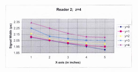
**Figure A.12** Signal width for Reader 2 located at (4,0,4). Tracking tag is on the elevated plane (z = 4). Observations were obtained for five points for each y-axis on the grid of the plane.
