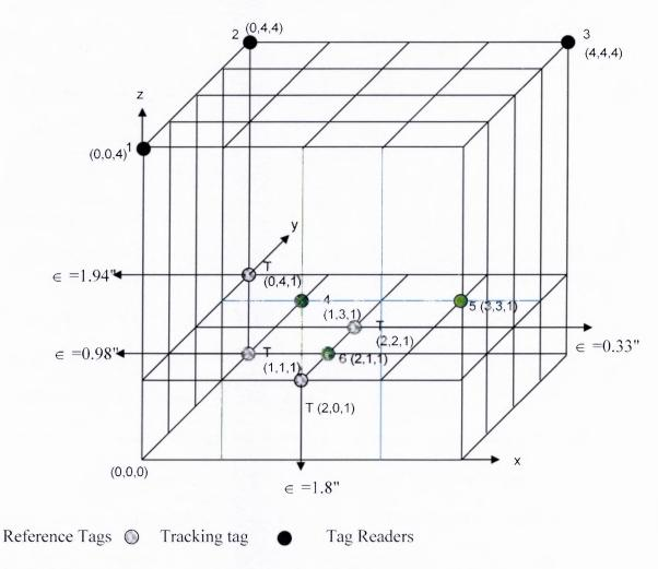
**Figure 4.2** Cube with three tag readers on top plane, reference tags and tracking tag on the elevated plane (z = 1). Error rates are shown for selected co-ordinates.
