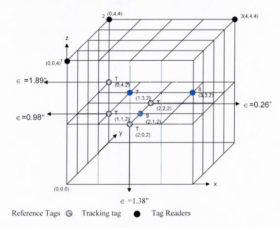
**Figure 4.3** Cube with three tag readers on top plane, reference tags and tracking tag are on the middle plane (z = 2). Error rates are shown for selected co-ordinates.
