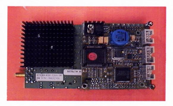
Figure 4.8 Tag-it<sup>TM</sup> reader module (RI-R00-320A).
