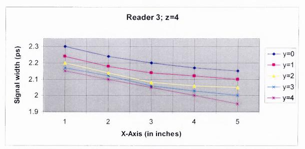
**Figure A.18** Signal width for Reader 3 located at (4,4,4). Tracking tag is on the elevated plane (z = 4). Observations were obtained for five points for each y-axis on the grid of the plane.
