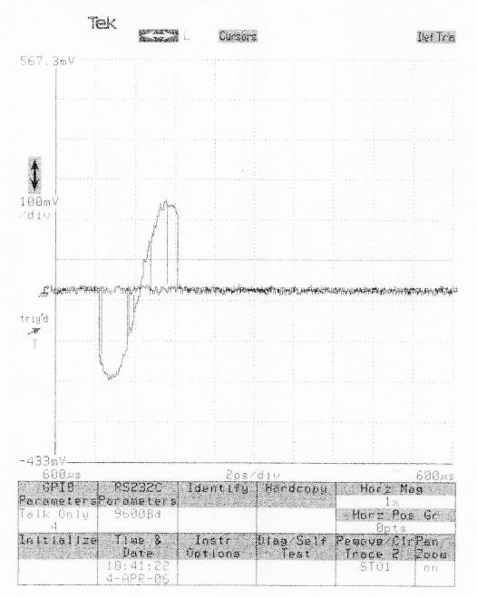
**Figure.4.15** A composite signal detected by an external antenna when a tag is placed at 0.1 inches from the reader's antenna (Signal width is 3.9 picoseconds).
