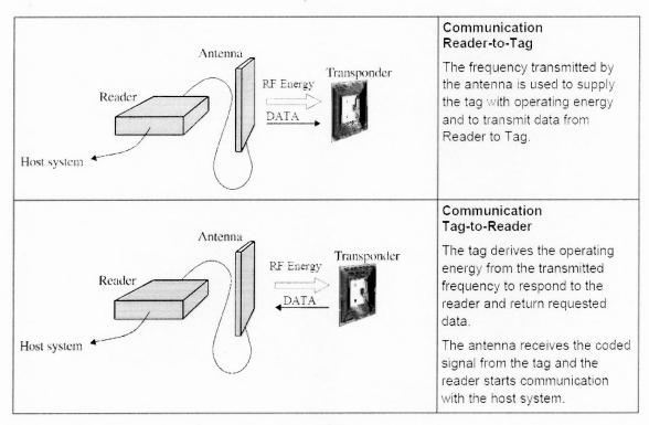
Figure 4.12 Communication modes of an RFID system.
