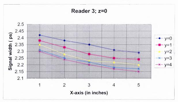
**Figure A.14** Signal width for Reader 3 located at (4,4,4). Tracking tag is on the lowest plane (z = 0). Observations were obtained for five points for each y-axis on the grid of the plane.
