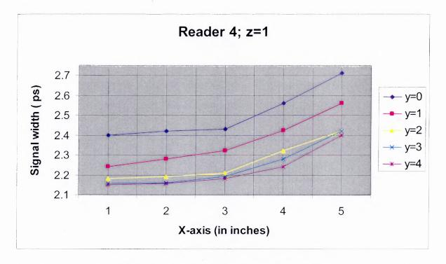
**Figure A.21** Signal width for Reader 4 located at (0,4,4). Tracking tag is on the elevated plane (z = 1). Observations were obtained for five points for each y-axis on the grid of the plane.
