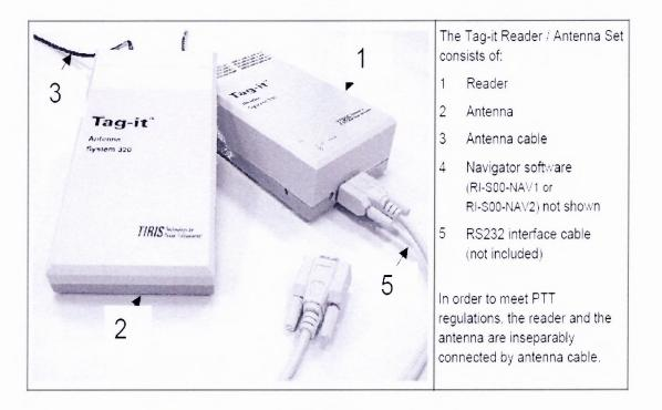
Figure 4.11 Tag-it<sup>TM</sup> reader / antenna set [19].
