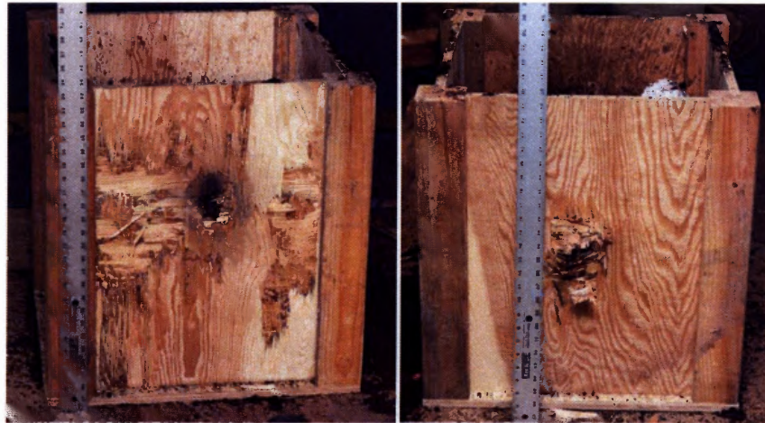
Figure 7.2 Damage of front panel (left) and back panel (right), caused by action of 230 g water-projectile in the first attempt.
