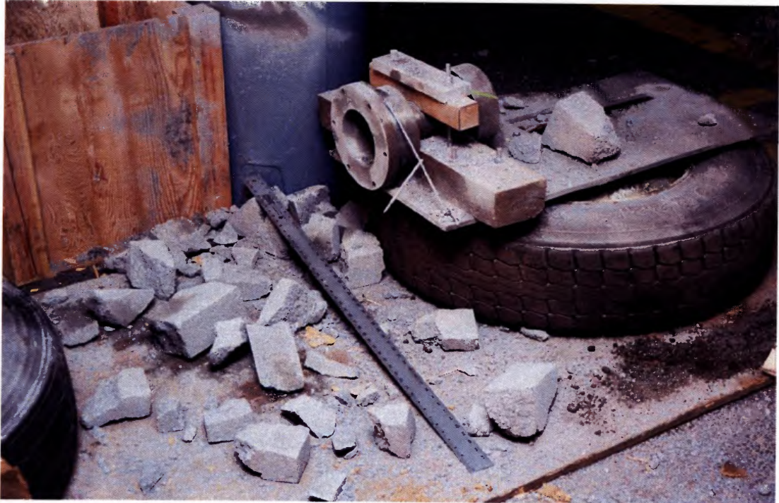
Figure 7.1.2 Concrete demolition caused by 230 g water projectile.
