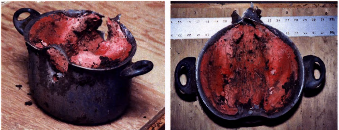
Figure 7.3 Damage of mine simulation unit caused by 230 g water-projectile in the first attempt.
