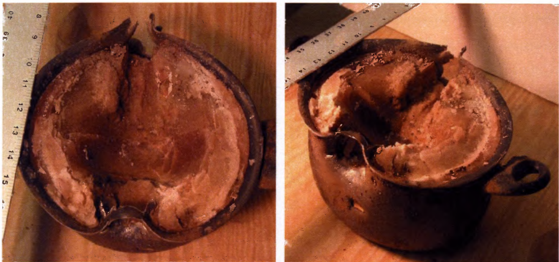
Figure 7.5 Damage of mine simulation unit caused by 230 g water projectile in the second attempt.
