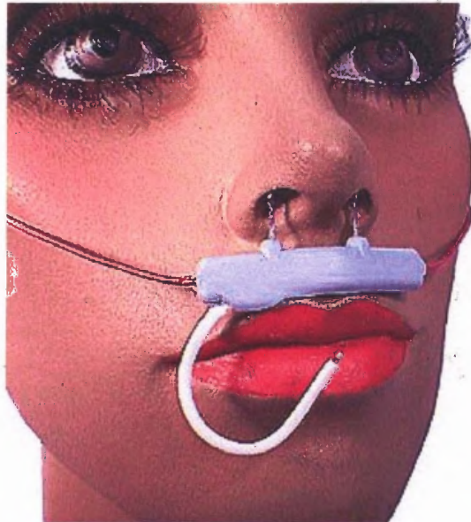
Figure 2.7 Thermistor sensor for respiration measurement [19].
