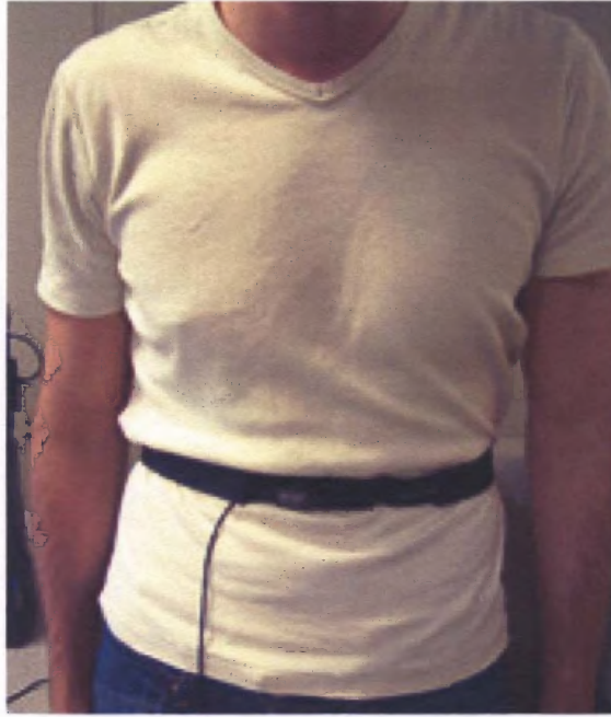
Figure 2.6 Displacement sensor for respiration measurement [17].
