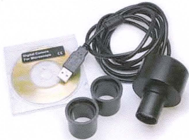
Figure 3.3 Digital eyepiece camera used in this experiment and referred as PC camera [12].
