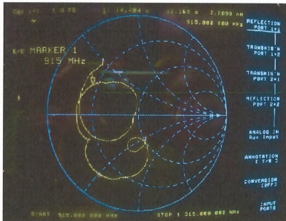
Figure 4.12 Smith Chart of Antenna Model-2 with integrated NIC-Cap(max)
