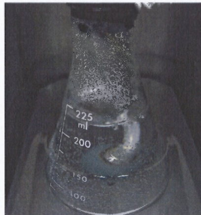
Figure 2.8 Erlenmeyer flask within heated water-bath. Gas is bubbled through sterile water for humidification prior to filtration and perfusion into culture chamber.
