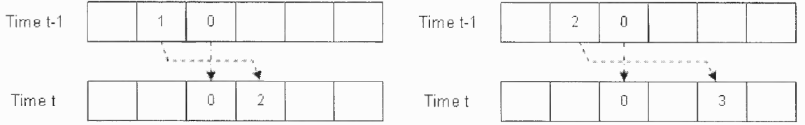
Figure 6.3 Invalid states in the DTMC-CA model. On a single lane road, the configurations at time t are not possible because they would involve vehicles crossing (or flying above) other vehicles.
