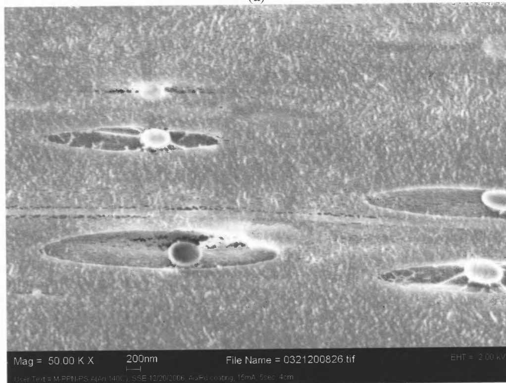
Figure. 3.41 SEM images of debonded morphology (50000X): (a) M-PP/PS, (b) M-PP/PS(An 140C).
