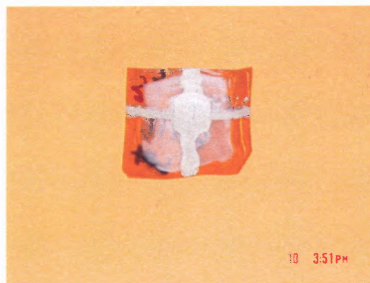
Figure 3.22 Pictures of the stencil printed silver top contact on Kapton.
