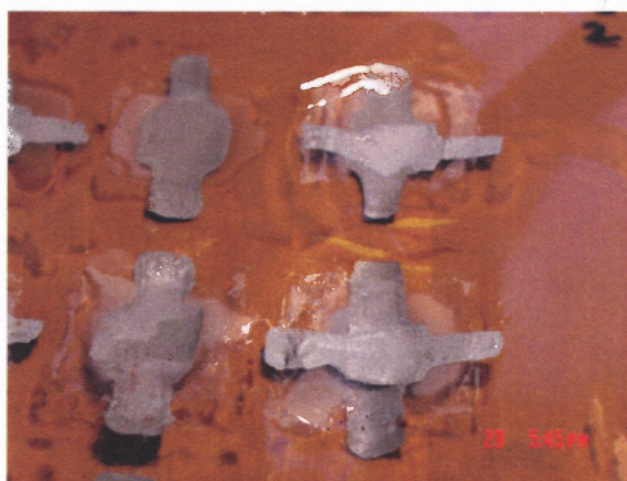
Figure 3.17 Pictures of the screen printed silver top contact on Kapton.
