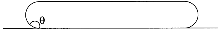
Figure 3.20 Equilibrium shape of droplets on the super-hydrophobic surface: (a) a droplet in capillary regime; (b) a droplet in gravity regime. \theta is the contact angle.
