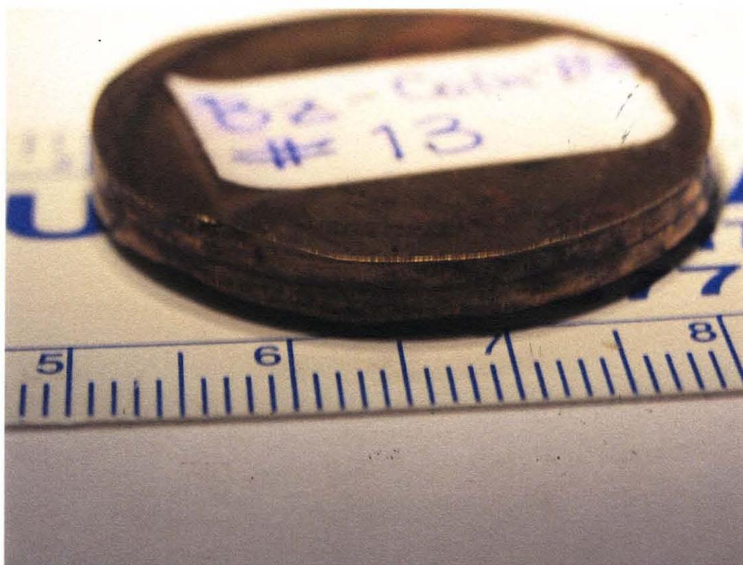
**Figure 10.9** General view of brass-nickel-alloy coin-brass plates welded by the water projectile impact in Exp. #13 at the water velocity 750m/sec.
