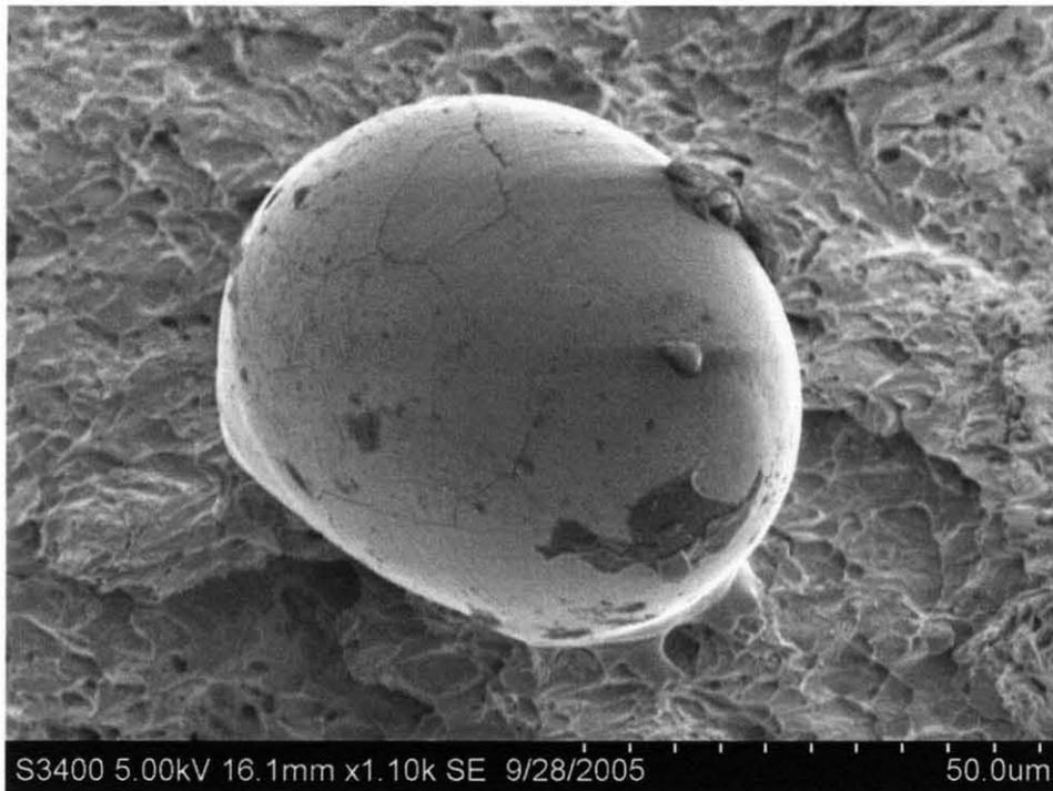
**Figure 5.3** SEM micrograph (X1100) of solidified egg like droplet formed in the final stage of steel failure.
