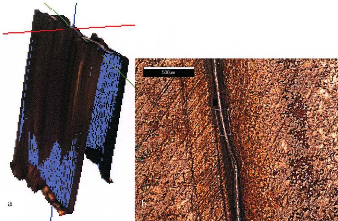
**Figure 8.4** a) Example of measurement of generated volume of extruded steel foil; b) 2-D view of extruded foil; inscribed polygon indicates projected area of measurement.
