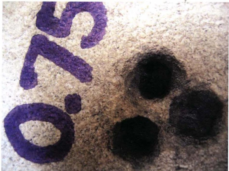
**Figure 11.15** Three impacts at the distance of  $\frac{3}{4}$ " between axes of impact zones. Notice minimal interference.
