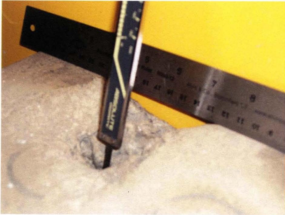
**Figure 11.12** Boring of granite by 52 sequential impacts. Notice dimensions of the generated cavity.
