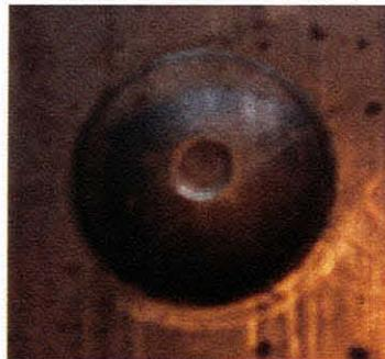
**Figure 6.25** Hemispherical dome is being formed during intermediate phase of forming process.
