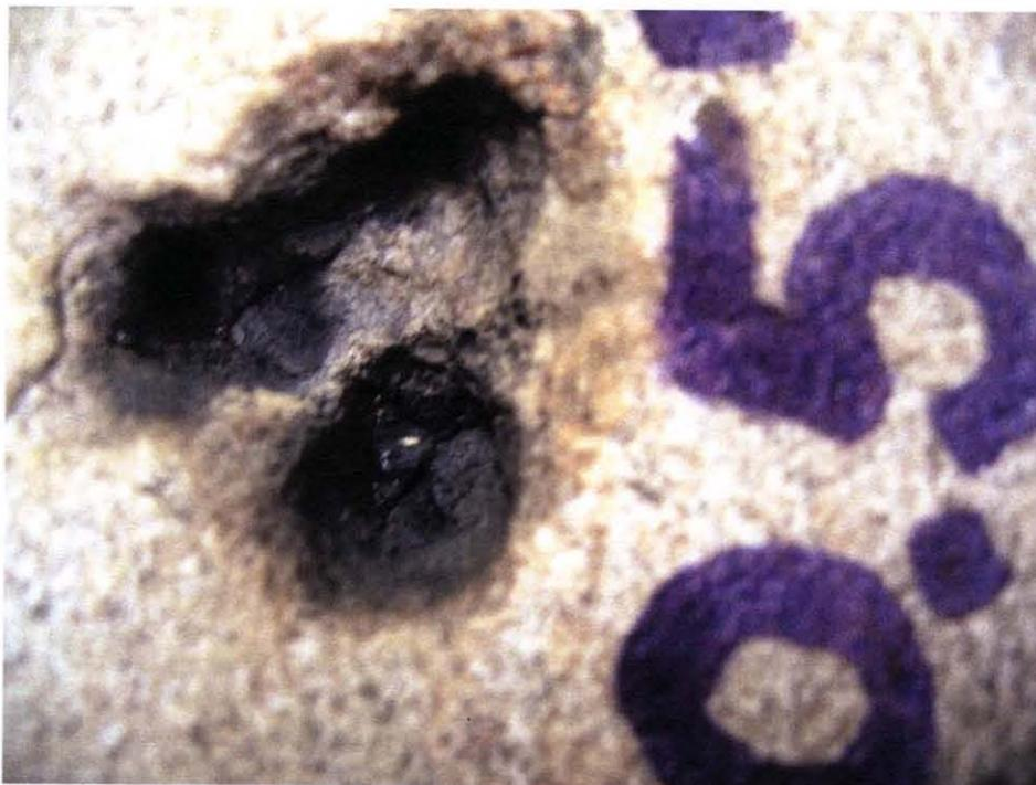
**Figure 11.16** Three impacts at the distance of  $\frac{1}{2}$ " between axes of impact zones. Notice significant interference between two shots.
