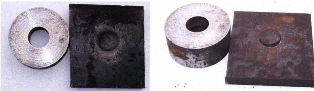
**Figure 6.14** Failed punching of 10mm thick steel plate against 16.5mm die diameter. Impacted and die side views.
