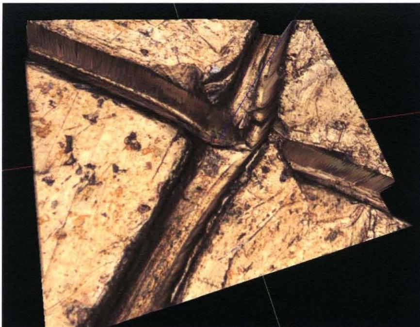
**Figure 7.18** Intersection of two micro channels formed on a brass sample by  $40\ \mu$  diameter tungsten wires.
