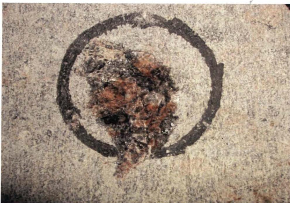
**Figure 11.19** Granite removal by impact of a projectile generated by low-power launcher.
