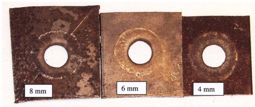
**Figure 6.7** Impact side views of punched openings in plates 8, 6 and 4mm thick. Punching was performed against die opening of 16.5mm in diameter.
