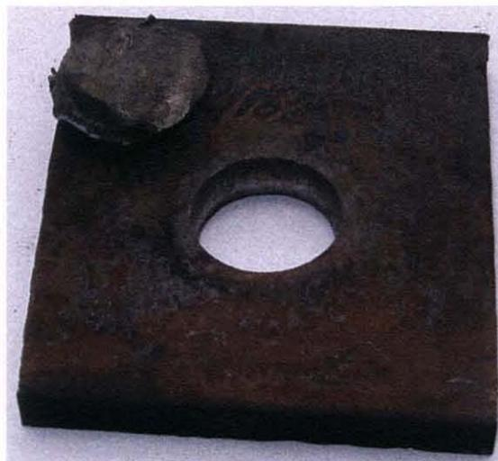
**Figure 6.6** A 10 mm thick plate with 25mm punched opening with punched part.
