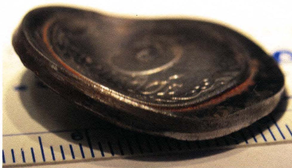
**Figure 10.22** General view of nickel alloy coin and steel plate welded by the water projectile impact at the water velocity 750m/sec (Exp.14, Table 10.1).
