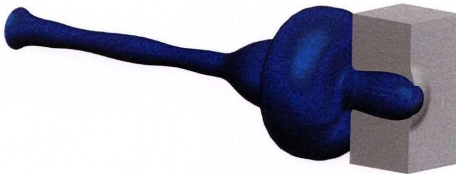
**Figure 5.10** Graphic representation of ductile hole growth mode of failure (see Fig 2.27).
