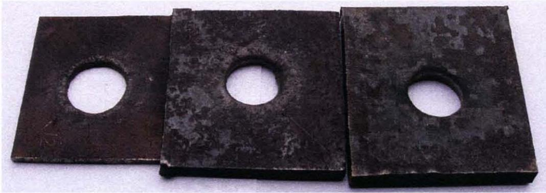
**Figure 6.4** Impact side views of punched openings in plates 4, 8 and 10mm thick. Punching was done against die opening 25mm in diameter.
