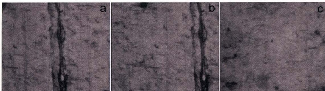
**Figure 9.3** Optical microscope images of areas tested on brass sample. a) inside track, b) next to track, c) control.
