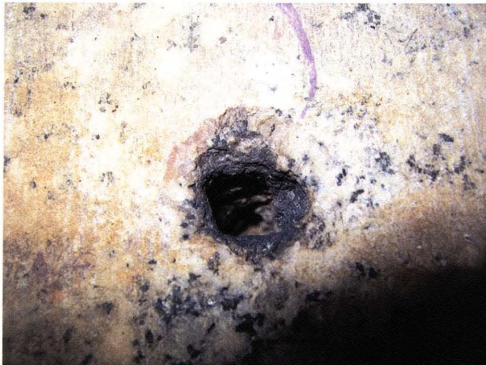
**Figure 11.11** Boring of a granite plate by sequential impacts of projectiles at the same site.
