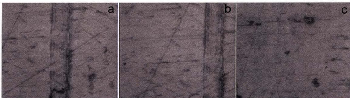
**Figure 9.5** Optical microscope images of areas tested on steel sample. a) inside track, b) next to track, c) control.
