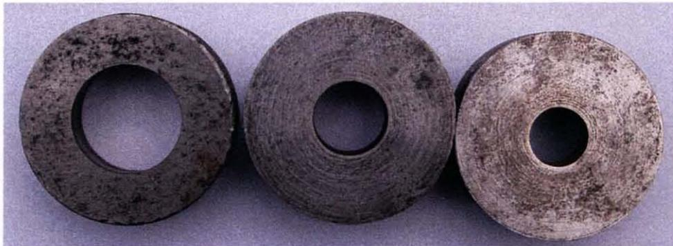
**Figure 6.3** Dies for punching of metals, diameters 25, 16.5 and 12mm.
