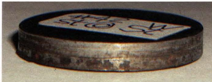
**Figure 10.17** General view of two steel plates welded by the water projectile impact at the water velocity 750m/sec (Exp. 42, Table 10.1).
