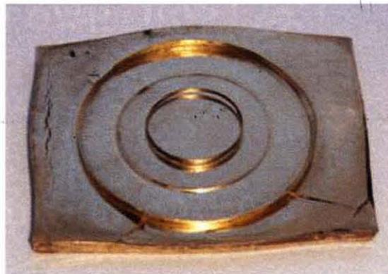
**Figure 7.30** Extruded circular brass rings.
