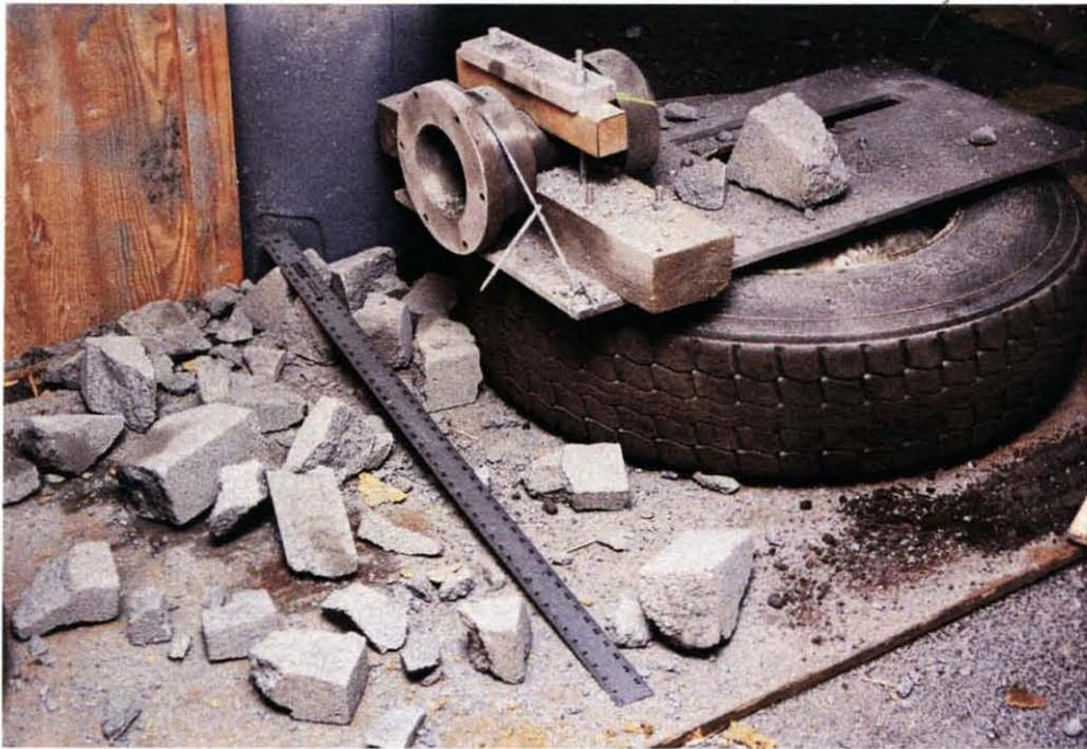
**Figure 5.15** Example of brittle fracture mode of failure (concrete demolition).
