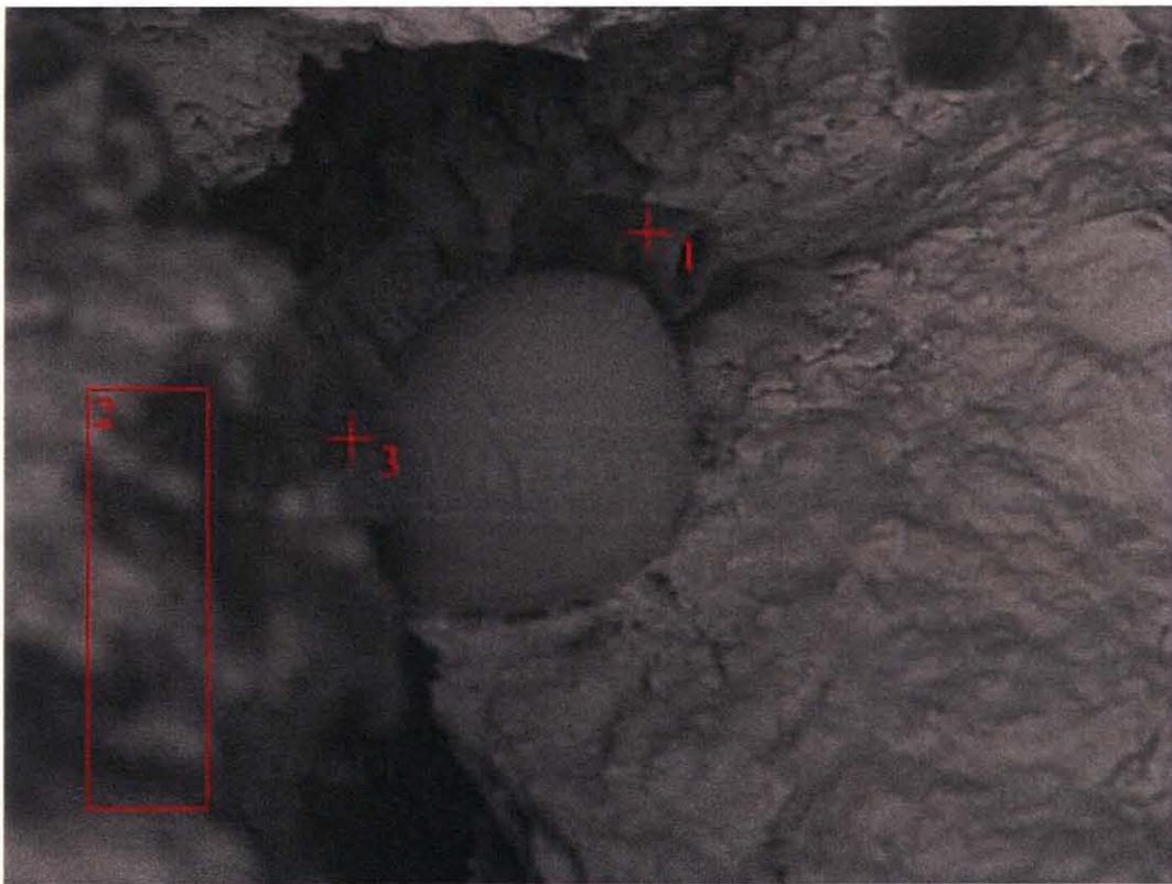
**Figure 5.5** SEM micrograph (X750) of solidified combination of egg like droplet and pipe like formed in the final stage of steel failure.
