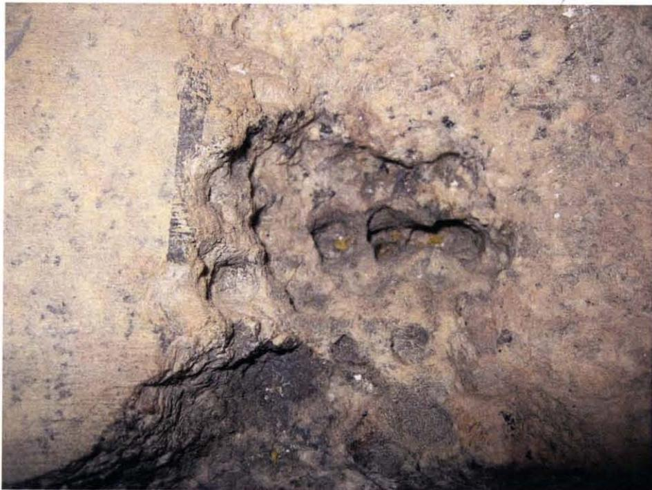
**Figure 11.13** Boring of granite by 52 sequential impacts.
