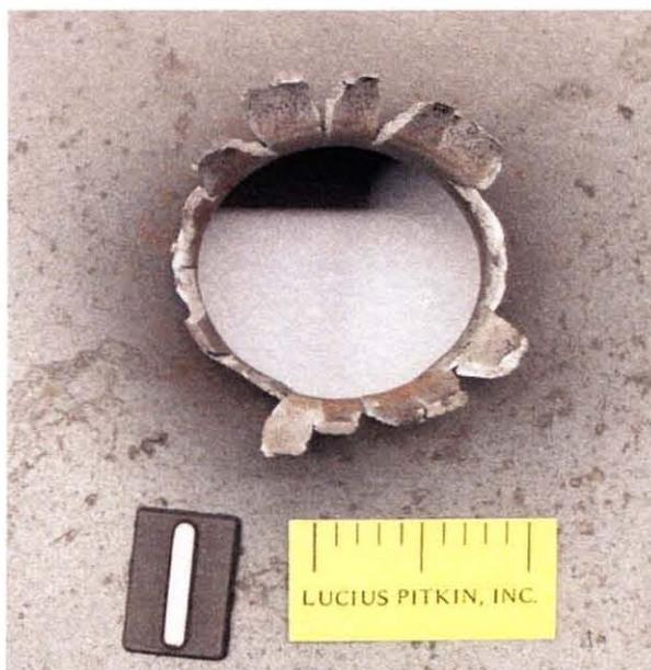
**Figure 5.1** General view of 4.8mm thick steel plate pierced by 230g water projectile.
