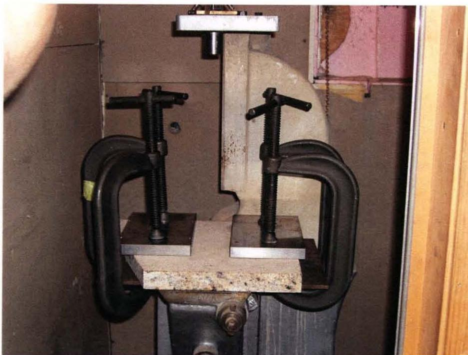
**Figure 11.18** Setup for granite boring at induced compressive stresses.
