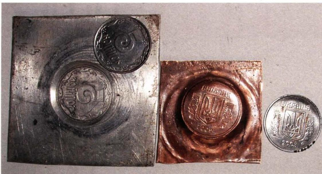
**Figure 7.12** General view of a coin stamped on aluminum and copper samples. Notice reproduction of fine details of the coin on the sample surface.
