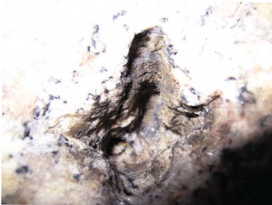
**Figure 11.17** Boring of a granite plate by sequential impact with a cross-like pattern of impact distribution.
