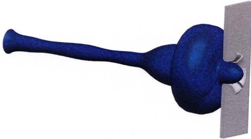
**Figure 5.14** Graphic representation of petaling mode of failure (see Figs. 4.2 and 5.1).
