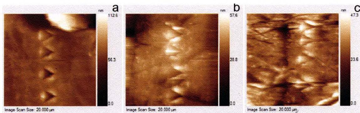
**Figure 9.4** SPM images after testing on brass showing residual indent impressions left on sample surface. a) inside track, b) next to track, c) control.
