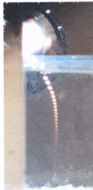
(c) Molten copper particle shooting through the water and cooling.
