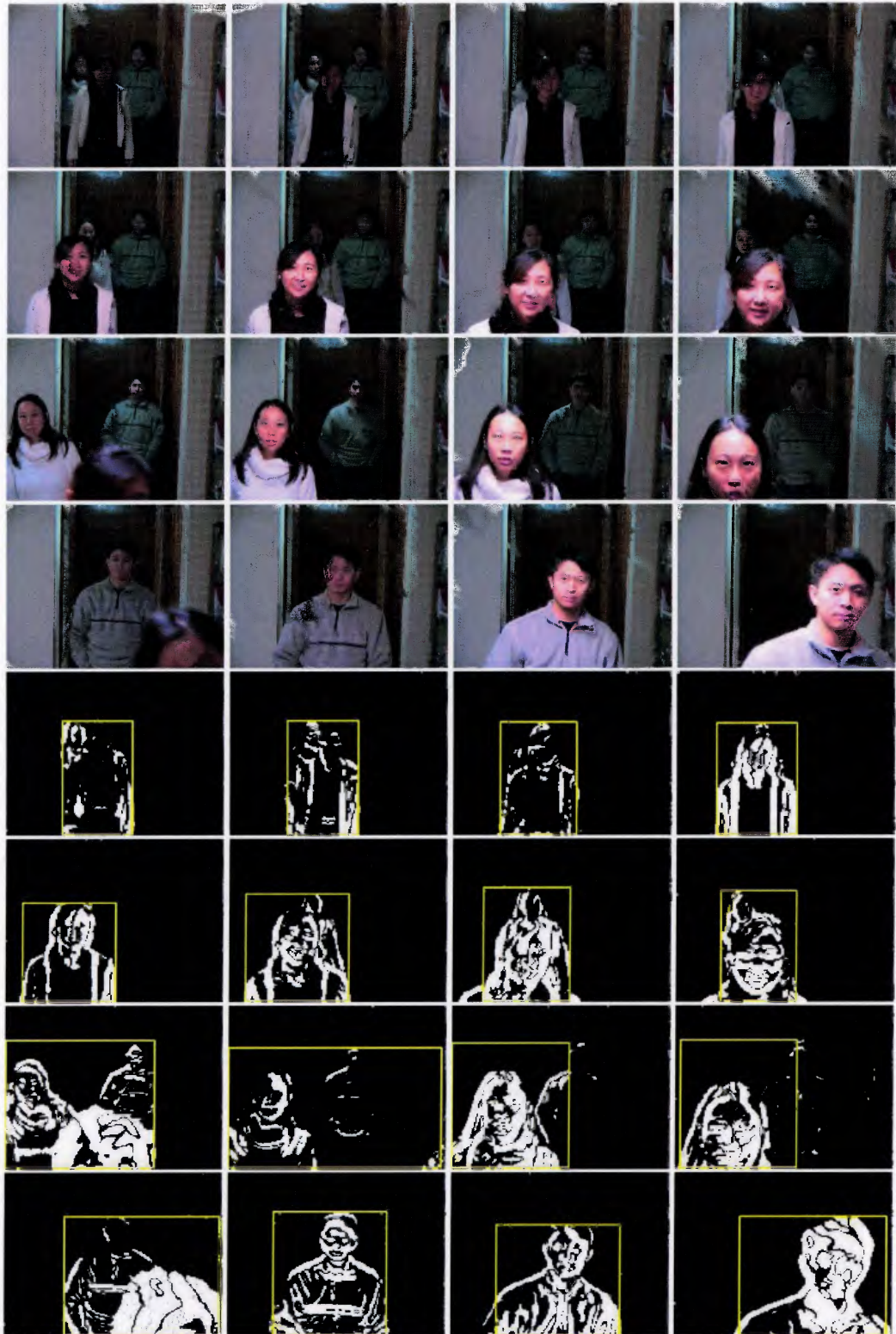
Figure 2.24 Face detection in a video stream with illumination variation. The upper half of frames show the original input stream, and the lower half of frames show the motion analysis results.
