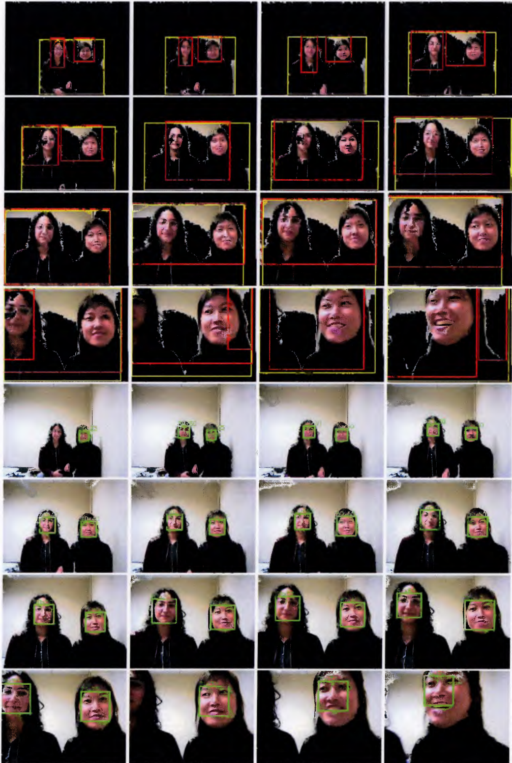
Figure 2.21 Face detection in a video stream. The upper half of frames show the FOIs derived from both motion analysis and skin color segmentation, and the lower half of frames show the face detection results.
