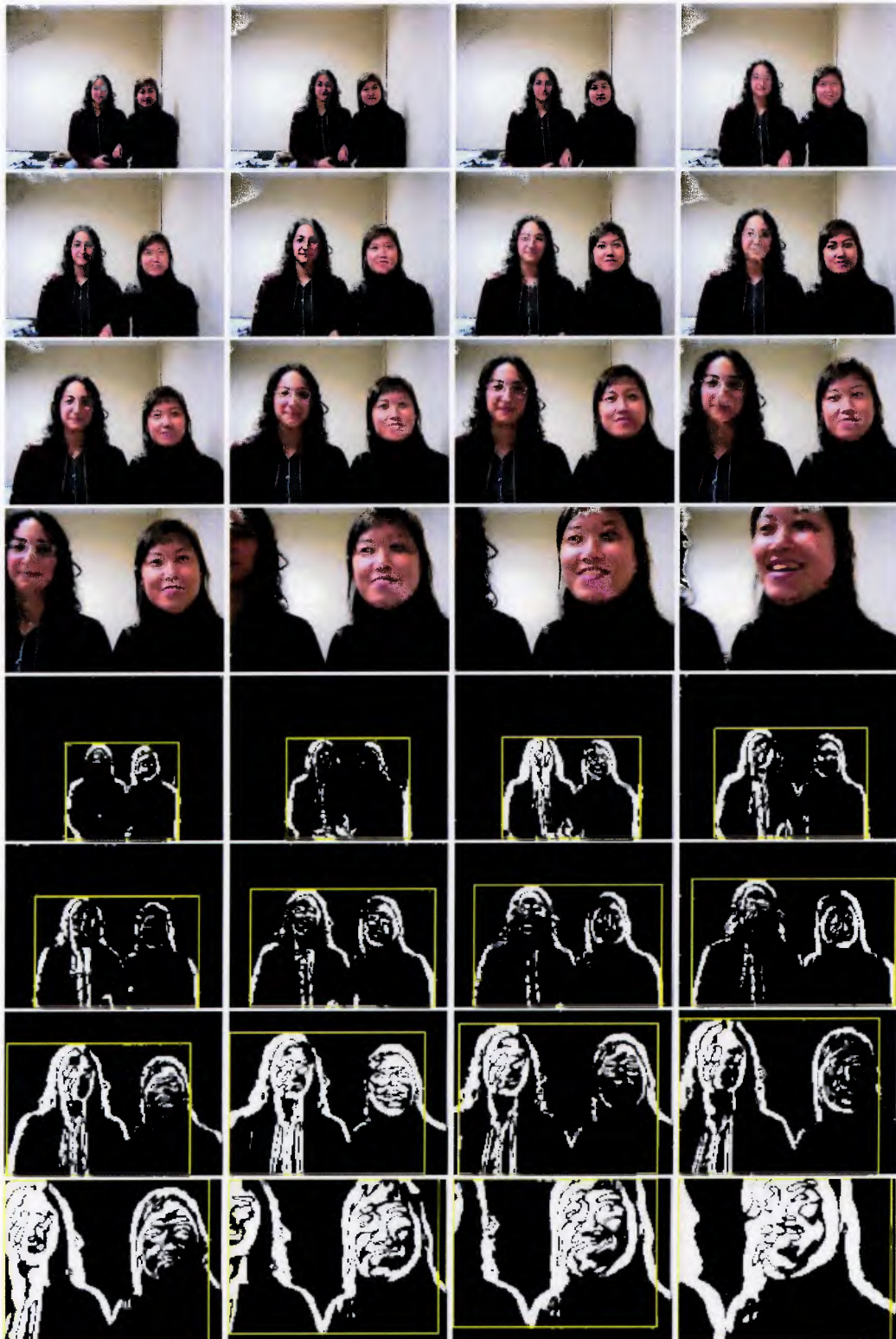
Figure 2.20 Face detection in a video stream. The upper half of frames show the original input stream, and the lower half of frames show the motion analysis results.
