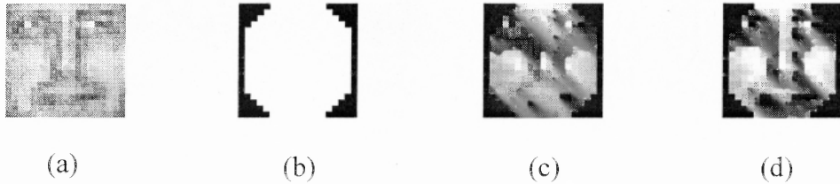
Figure 3.1 Face image preprocessing. (a) Original face image, (b) the mask, (c) normalized image, and (d) histogram equalized image.
