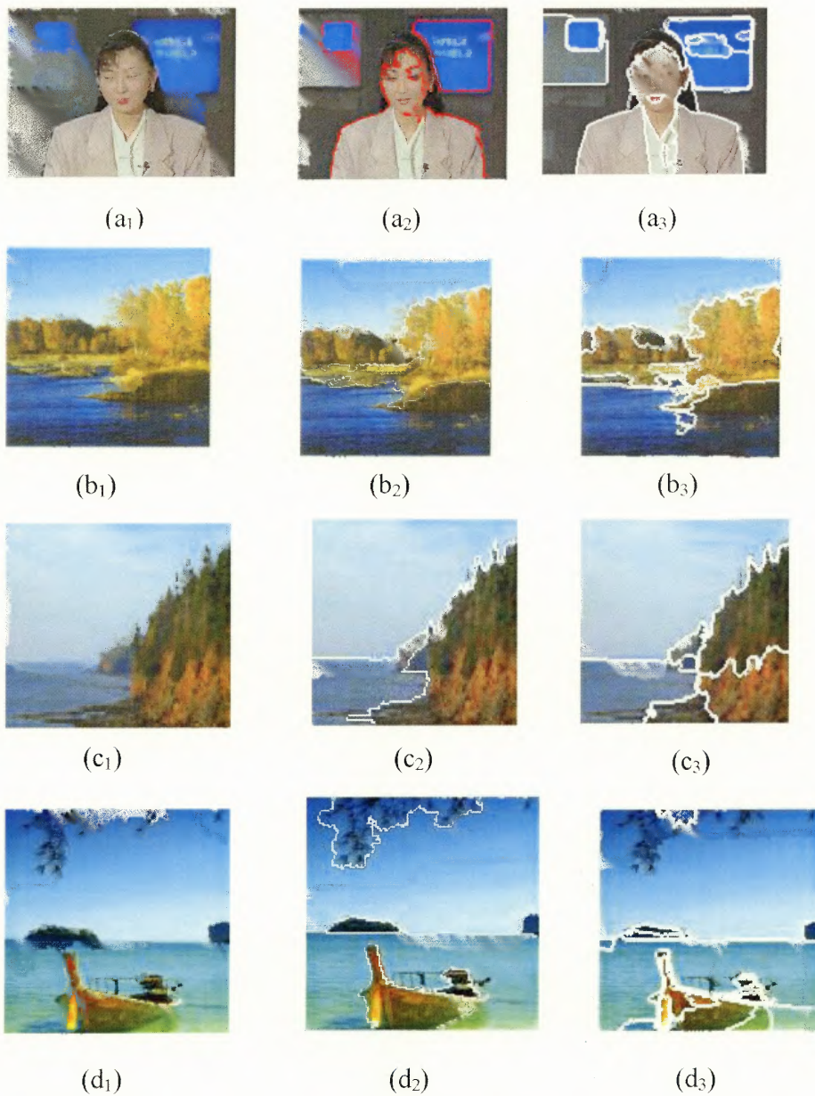
Figure 2.1.8 The first column shows the original images, the second column shows the segmented results of the proposed SRG method, and the third column shows the results of Fan's algorithm.
