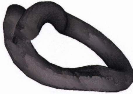
Figure 4.5 Badly rendered self-intersecting generalized swept surface.
