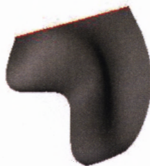
Figure 3.7 Non-periodical critical swept surface of a line segment.
