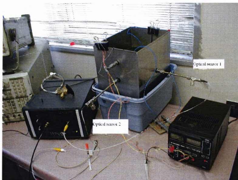
Figure 5.6 Two dimensional localization of PD experiment setup.
