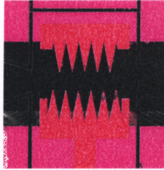
Figure A.8 Mechanical Shearing Device, Polysilicon Teeth.
