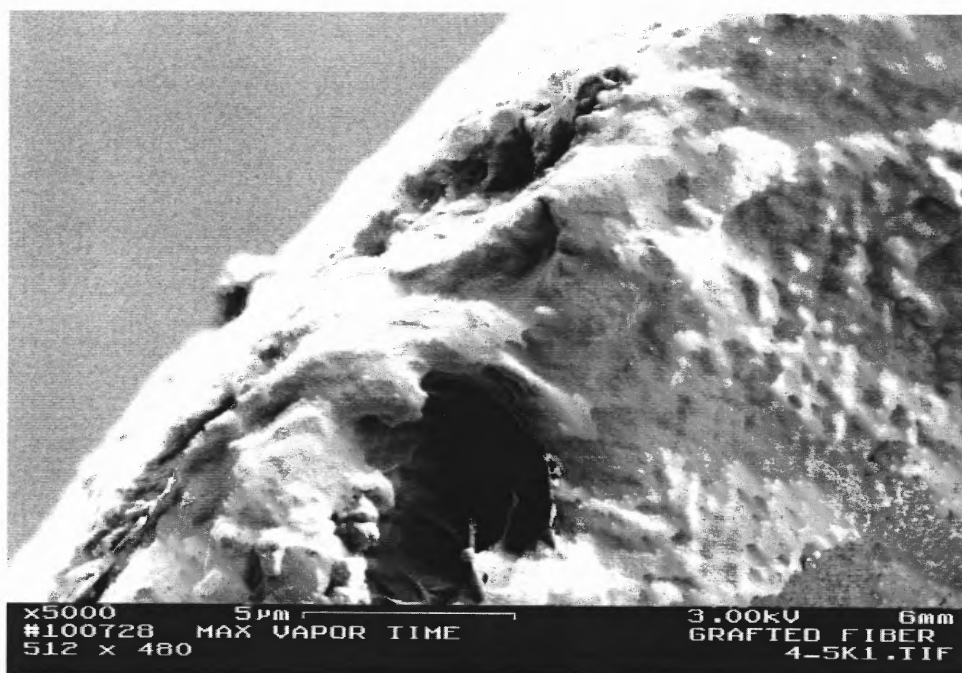
Figure 3.10. Cross-sectional view of the AA-grafted hollow fiber from Batch 4: High Graft Exposure Time.
