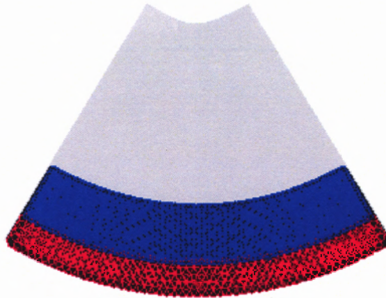
Figure 7.8 Setting of binary particulate bed before simulation.
