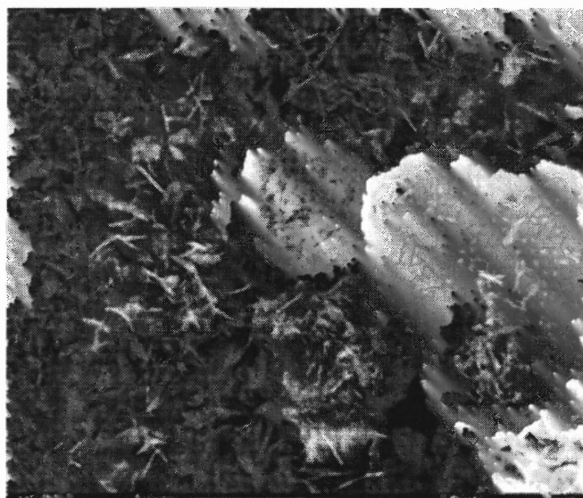
Figure 6.2 Hydroxide formation on the surface of as-received magnesium after 100 hours of exposure to atmosphere.
