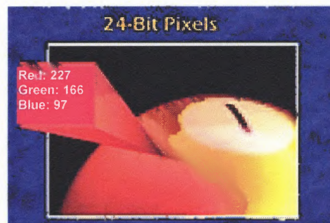
Figure 5.3 The Color Intensity in One Pixel of the 24-Bit Pixel Image (Kodak, 2002).
