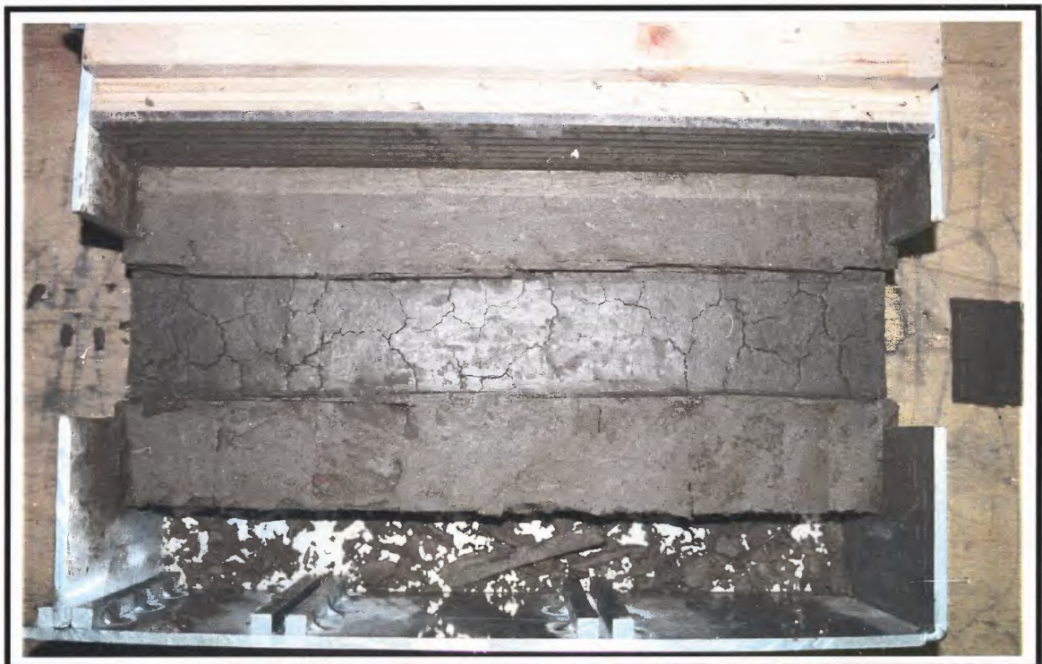
Photograph A-14. A similar form of shrinkage cracking occurred on the lower surface of the fracture.
