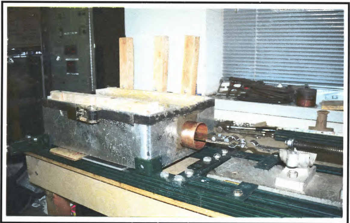
Photograph A-8. The sheet metal spacer was pulled from the soil using a modified sample ejector leaving an open discrete fracture.
