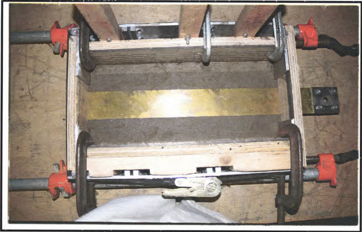
Photograph A-7. The sheet metal spacer is placed on top of the compacted soils. Note the slightly slickensided surface.
