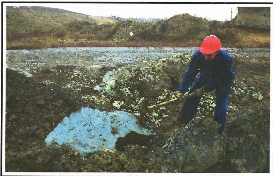
Photograph A-4. The clay maintained itself as large blocks and was difficult to breakdown.
