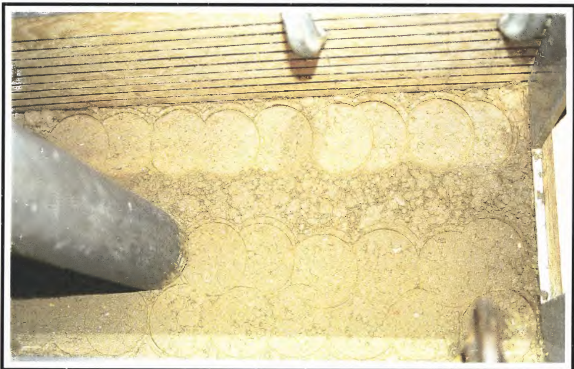
Photograph A-6. The clay was compacted using a series of blows from a Proctor rammer.
