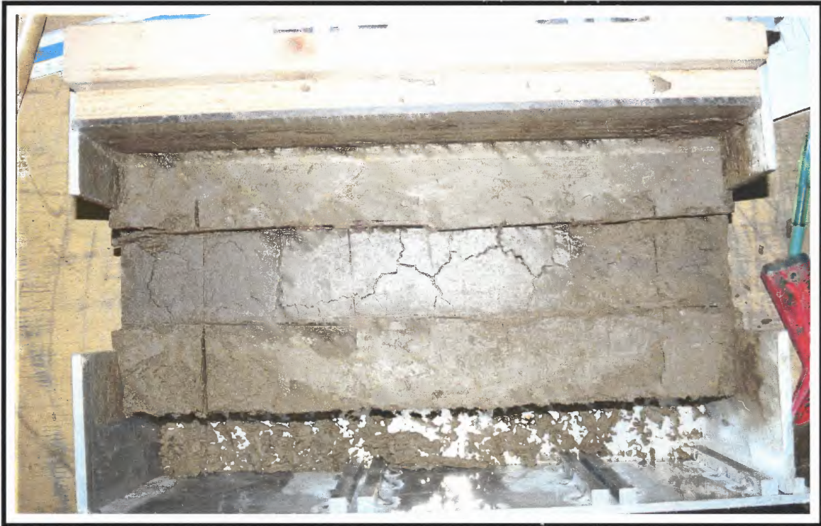
Photograph A-15. Wetting caused preferential swelling at the inlet end (on right). Others parts of the fracture were representative of drying conditions.
