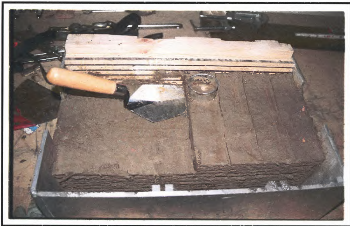
Photograph A-11. The soil block was excavated and sampled in vertical and horizontal layers to obtain moisture data.
