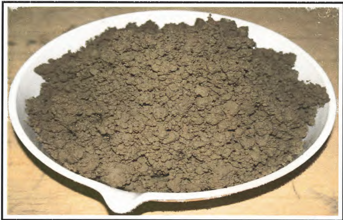
Photograph A-5. This photograph shows the form of the soil clods prior to compaction. The diameter of the bowl is approximately 10 inches.
