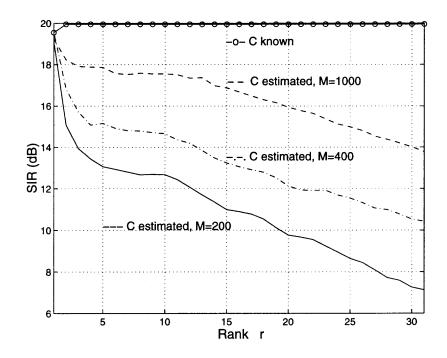
Figure 2.2 SIR of the MMSE detectors. N=31, K=10, SNR=20dB, (K-1) interferences' SNRs 10dB.
