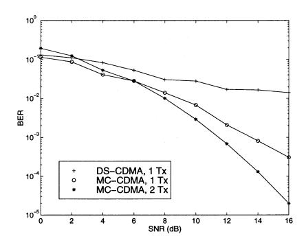
Figure 3.2 BER versus SNR for DS-CDMA, MC-CDMA with one antenna and with two antennas,  $\mathrm{K}{=}10$
