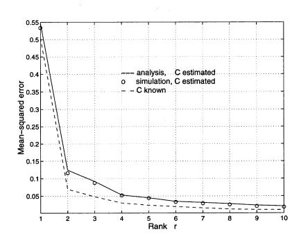
Figure 2.7 MSE of the MMSE detectors. N=31, K=10, SNR=20dB, K-1 interference users' SNRs are 16dB, 17dB, 18dB, 19dB, 20dB, 21dB, 22dB, 23dB, 24dB.
