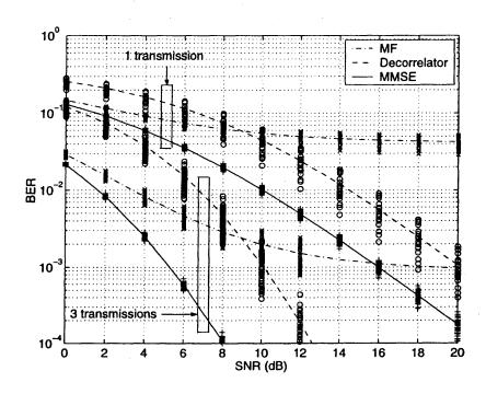
Figure 4.1 BER versus SNR for the slotted CDMA system.  $\alpha = 3/8$ , L = 2, Processing gain N = 64 in simulation.
