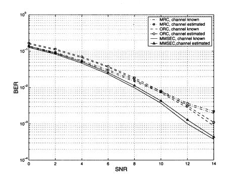
Figure 3.12 Bit error rate of MC-CDMA with pilot symbols.  $f_dT_b = 0.001$ , K=10, P=6dB, M=4
