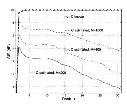
Figure 2.3 SIR of the MMSE detectors. N=31, K=10, SNR=20dB, (K-1) interferences' SNRs are 10dB, 10dB, 10dB, 10dB, 10dB, 20dB, 30dB, 30dB, 40dB.
