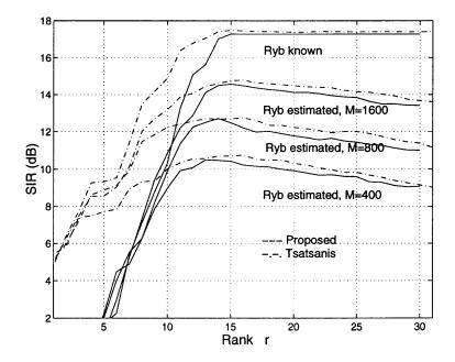
Figure 2.11 Output SIR comparison for different ranks. N=31, K=8, SNR=20dB, (K-1) interferences' SNRs are 30dBs.
