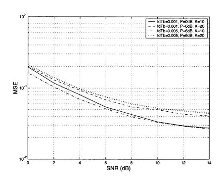
Figure 3.6 Mean squared-error of the channel estimator using pilot channels.
