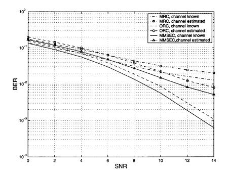
Figure 3.15 Bit error rate of MC-CDMA with pilot symbols.  $f_dT_b = 0.005$ , K=20, P=9dB, M=2
