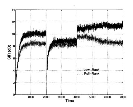
Figure 2.12 Performance of the adaptive reduced-rank MMSE detector in a dynamic multiple-access channel.
