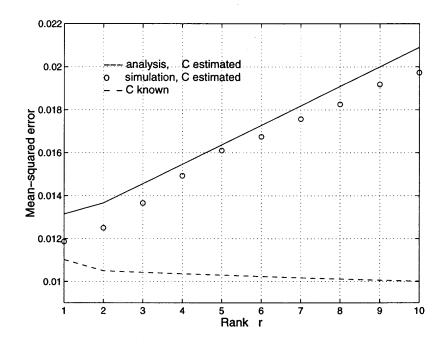
**Figure 2.5** MSE of the MMSE detectors. N=31, K=10, SNR=20dB. K-1 interference users' SNRs are 8.4dB, 8.8dB, 9.2dB, 9.6dB, 10dB, 10.4dB, 10.8dB, 11.2dB, 11.6dB.
