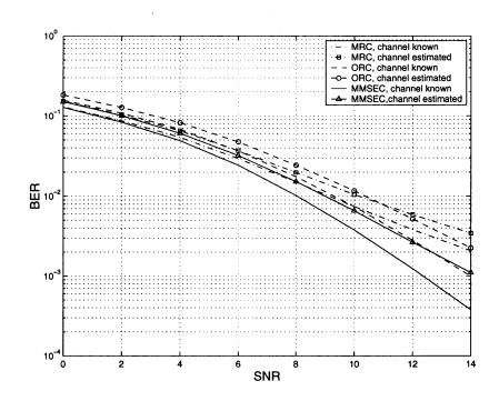
Figure 3.14 Bit error rate of MC-CDMA with pilot symbols.  $f_dT_b = 0.005$ , K=10, P=9dB, M=2
