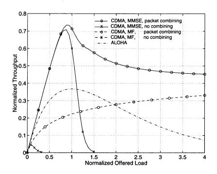
Figure 4.5 Normalized throughput of the slotted CDMA system. SNR = 20dB, L = 2.
