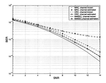
Figure 3.13 Bit error rate of MC-CDMA with pilot symbols.  $f_dT_b = 0.001$ , K=20, P=6dB, M=4
