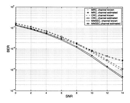
Figure 3.7 Bit error rate of MC-CDMA with pilot channels.  $f_dT_b = 0.001$ , K=10, P=0dB.
