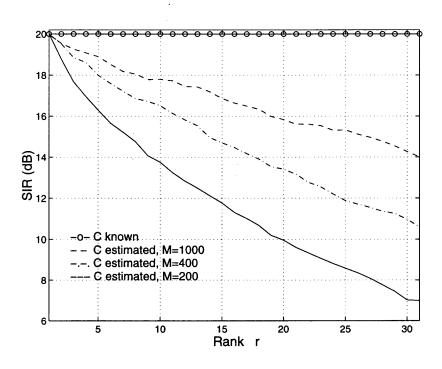
Figure 2.1 SIR of the MMSE detectors. N=31, K=1, SNR=20dB.
