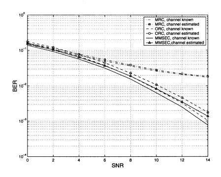
Figure 3.10 Bit error rate of MC-CDMA with pilot channels.  $f_dT_b = 0.005$ , K=20, P=6dB.
