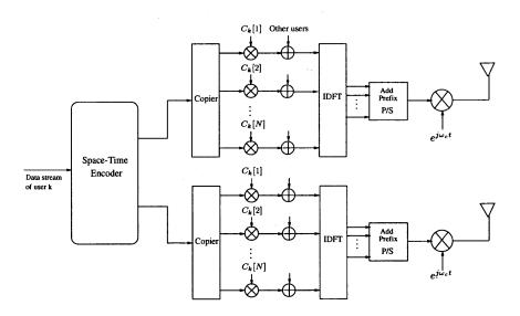
Figure 3.1 A MC-CDMA transmitter with transmit diversity
