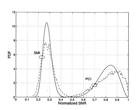
Figure 2.13 Density function of normalized output SNR, input SNR=15dB, M=400, N=31, p=4.
