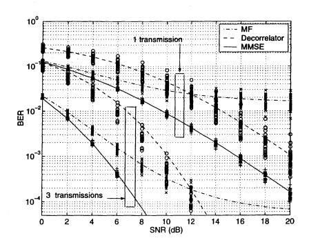
Figure 4.2 BER versus SNR for the unslotted CDMA system.  $\alpha = 3/16, L = 2$ , Processing gain N = 64 in simulation.
