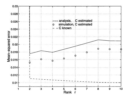
Figure 2.6 MSE of the MMSE detectors. N=31, K=10, SNR=20dB. K-1 interference users' SNRs are 8dB, 9dB, 10dB, 11dB, 12dB, 20dB, 30dB, 31dB, 40dB.
