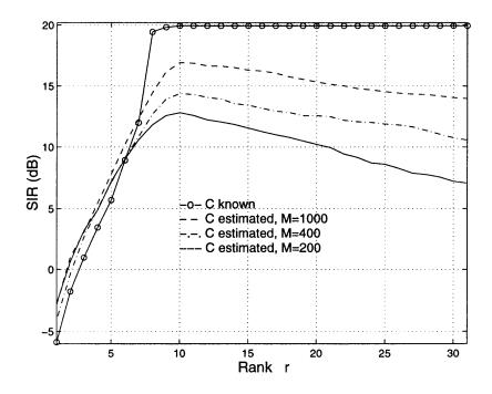
Figure 2.4 SIR of the MMSE detectors. N=15, K=10, SNR=20dB, (K-1) interferences' SNRs are 20dBs.
