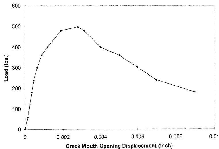
Figure 5.30b Load-CMOD Relationship of Beam JS1 (Jenq and Shah 1985)
