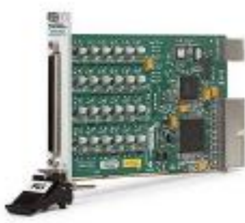
Figure 3.8 NI PCI 6259 DAQ Board, maximum sampling frequency is 1.25 MHz.
