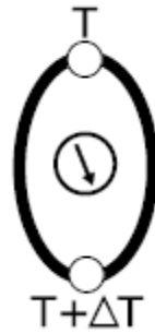
Figure 2.2 The experimental device used by Seebeck to discover the first thermoelectric effect.
