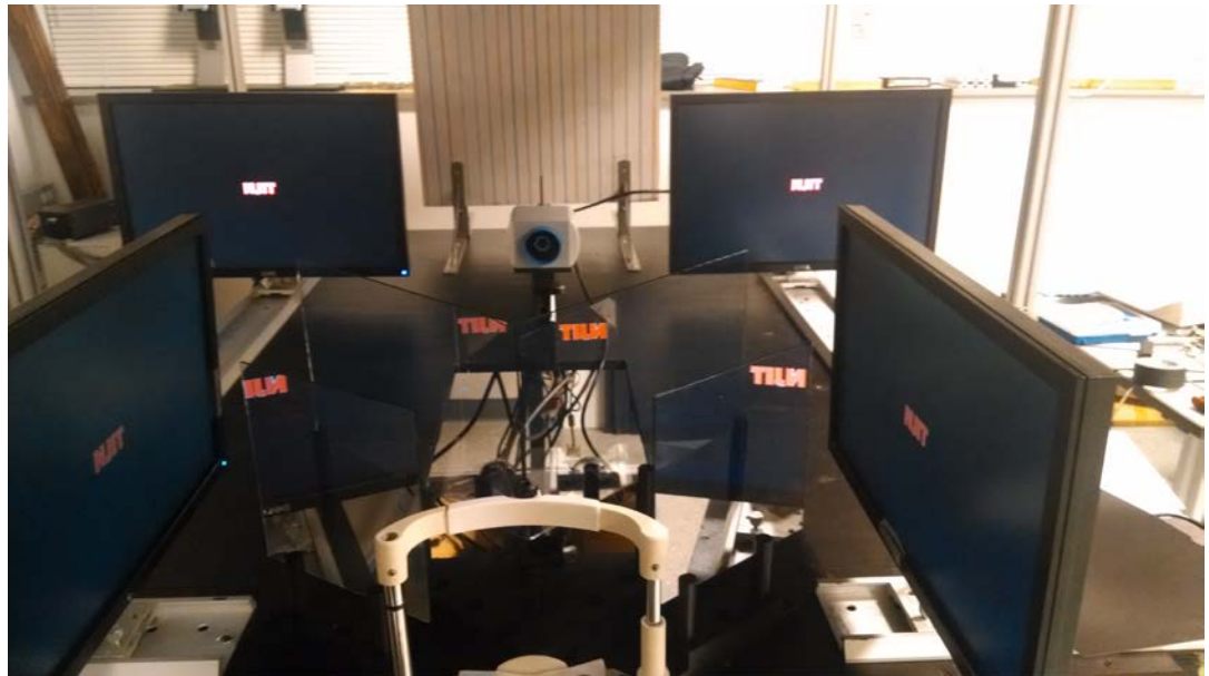
Figure 7 Power Refractor III as installed in Haploscope. Based upon the manufacturer's recommendation the system is automatically calibrated so long as it is 1m away from the subject.
