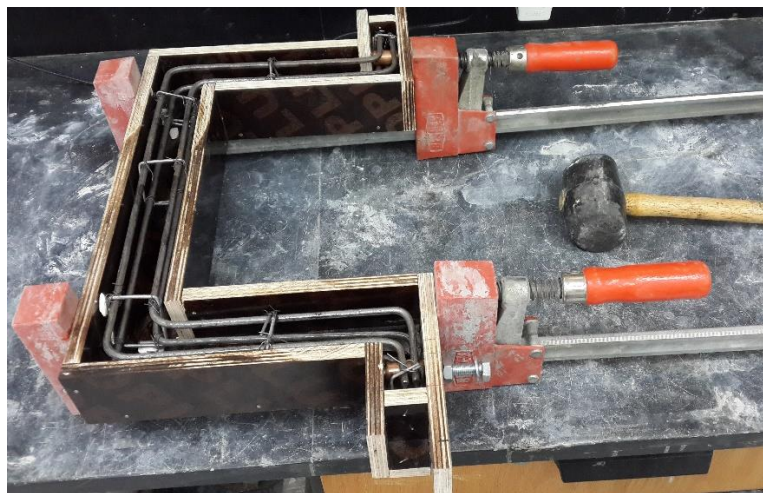
Figure A.2 The wood works and reinforcement for the RC frame.
