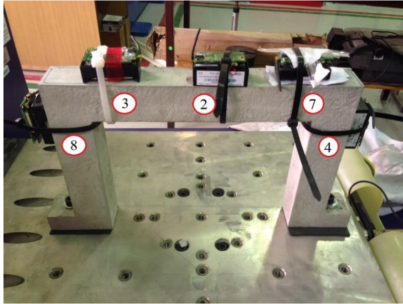
Figure 3.4 Wireless sensors arrangement mounted on RC frame.
