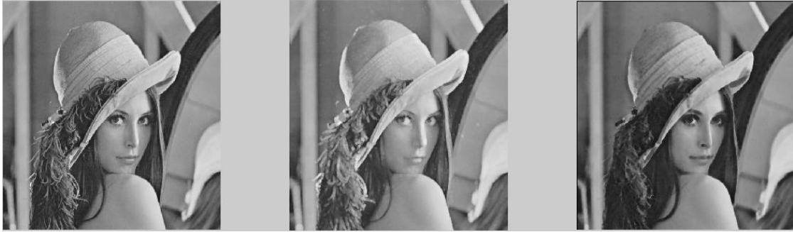
Figure 3.2 Comparison of original, dilated and eroded Lena images.
