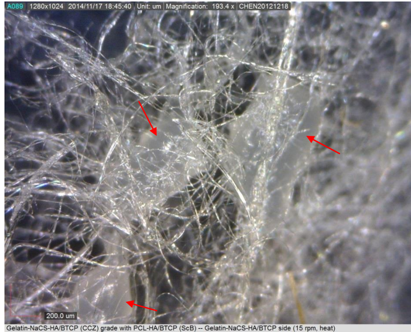
Figure 3.15 Light microscope image of the Gelatin-NaCS-HA/ \beta -TCP side of the PCL-HA/ \beta -TCP //Gelatin-NaCS-HA/ \beta -TCP scaffold after heating 5 hours at 150°C. Aggregates are visible.
