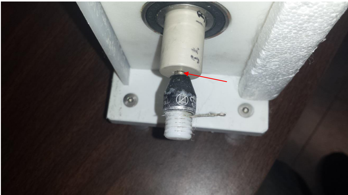
Figure B.3 Close up of the uncovered slip ring. The metallic portion of the slip ring (arrow) contacts the wire that runs from the mandrel in Figure B.2. A small eye hook protrudes from the slip ring (this hook contacts the underlying metal in the slip ring), which allows for the connection of the grounding wire.
