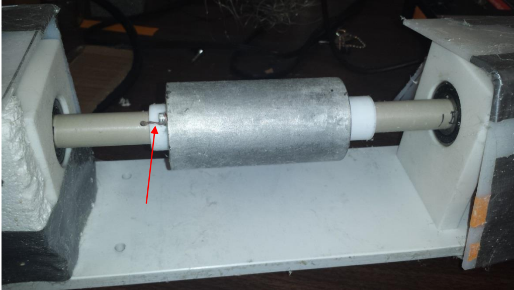
Figure B.2 Close up of mandrel collection plate. A small wire attaches to the side of the metal plate and runs through an insulated cylinder which connects to a slip ring on the left (covered in this photograph).
