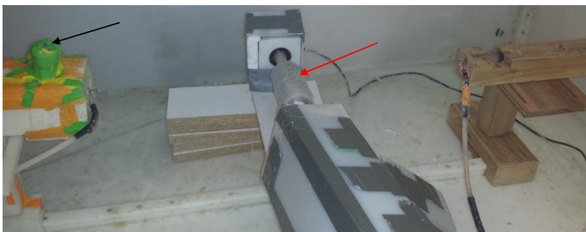
Figure 2.1 Picture of electrospinning setup. Left – polyethylene syringe holder which holds the gelatin based solutions. This syringe holder is housed within a Styrofoam housing to maintain a constant air temperature. The heated air line is fed through the hole in the top (arrow). Right – wooden syringe holder containing the PCL based solution. Middle – rotating mandrel with motor and slip ring ground connection covered by polyethylene sheets. The collection plate is identified by a red arrow. Note: the infusion pumps and voltage sources are not shown in this picture.
