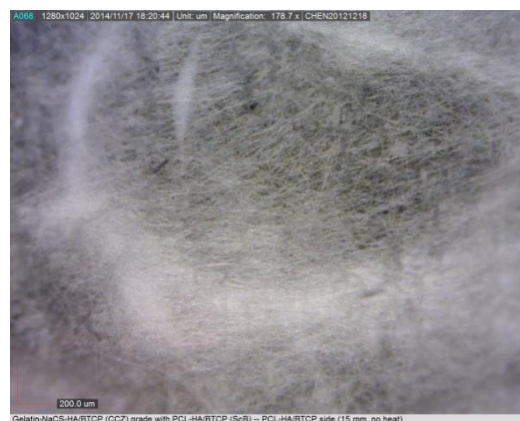
Figure 3.19 (A) Gelatin/PCL scaffold with mandrel at 2300rpm, (B) Gelatin/PCL scaffold with mandrel at 4200rpm, and (C) the CCZ/SCB scaffold previously discussed which was electrospun onto a 15rpm mandrel.
