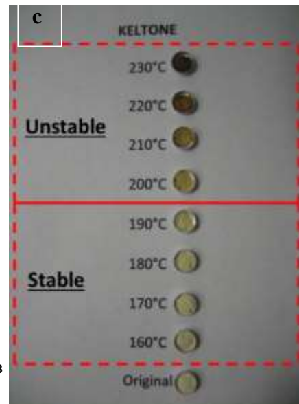
Figure 4.3 (a) Ramp heating of Keltone under air, (b) isothermal heating for 10 min, (c) degradation-induced color change relative to the original material.
