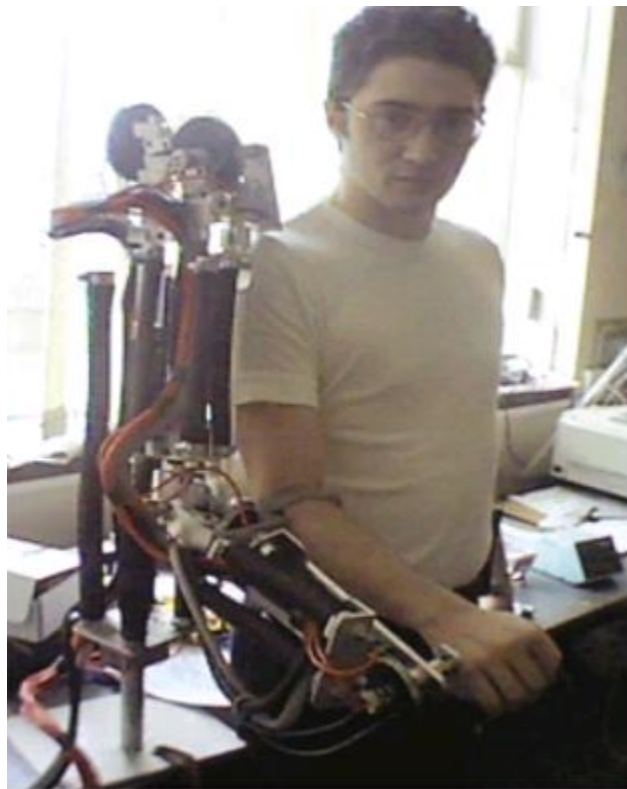
Figure 2.9 Exoskeleton prototype using pneumatic Muscle Actuators (pMA) attached to a person's arm.
