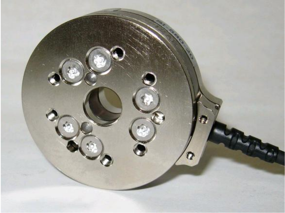
Figure 3.2 ATI Industrial Automation Mini45 Force Transducer. Source: [38]
