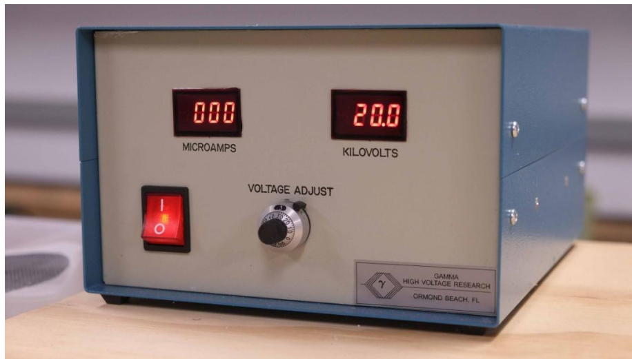
Figure 2.4 High Voltage supply.
