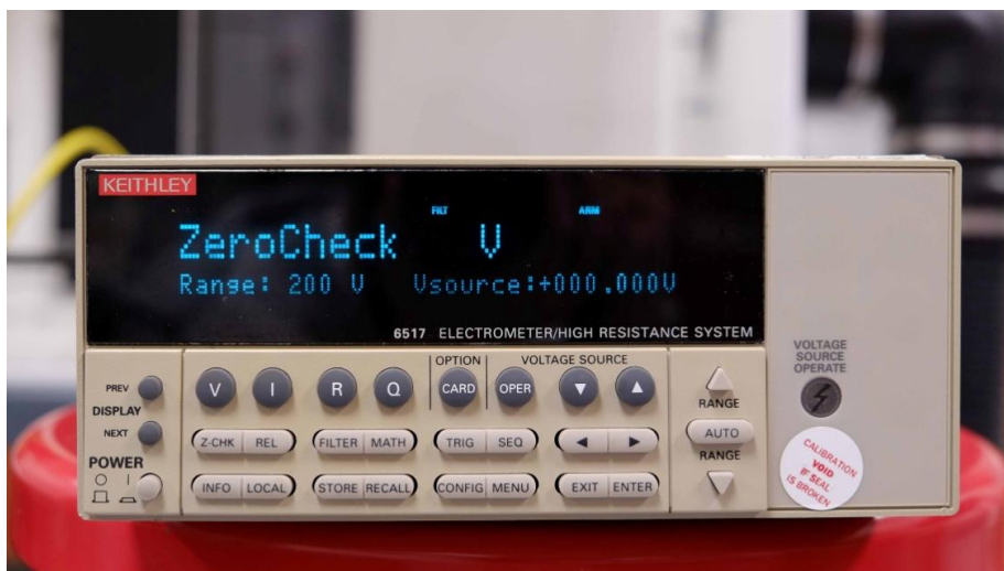
Figure 2.6 Programmable electrometer used for current measurement in the electrospinning process.
