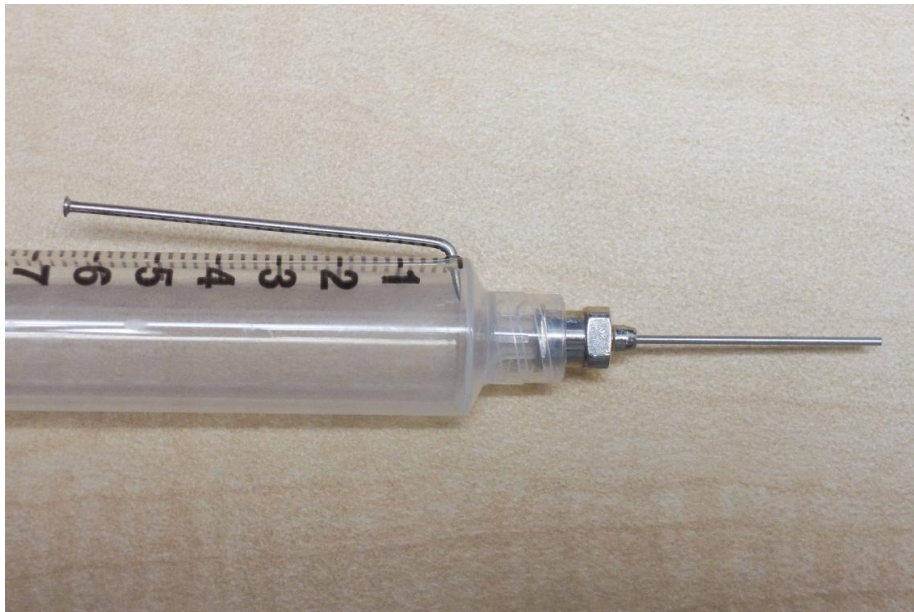
Figure 2.7 Modified syringe assembly used for electrospinning process.
