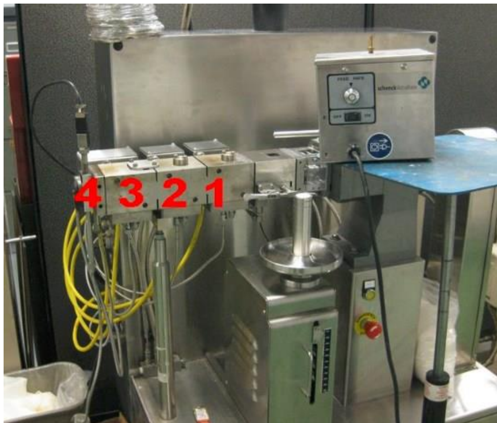
Figure 3.4 The Leistritz's Nano 16 Twin-Screw Extruder (the numbers shown in the picture denote the four heated barrel zones).
