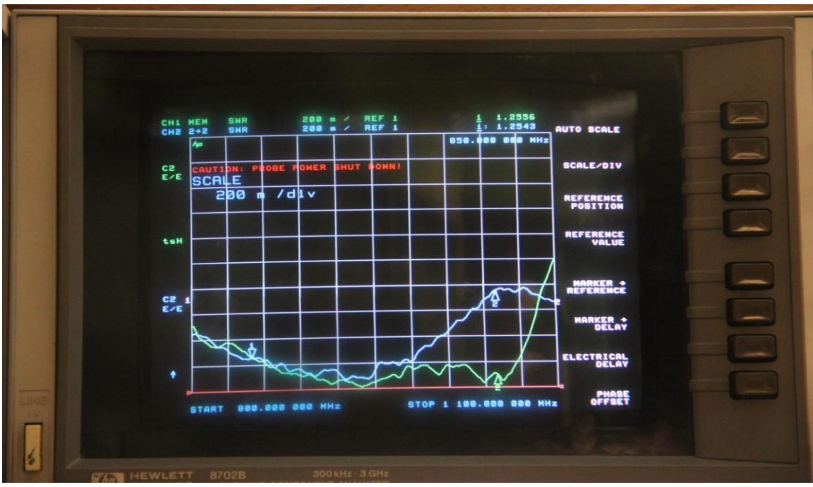
Figure 4.19 VSWR measurement for new bent bow tie RFID antenna (green) and Poynting Patch A 0025 antenna (blue).
