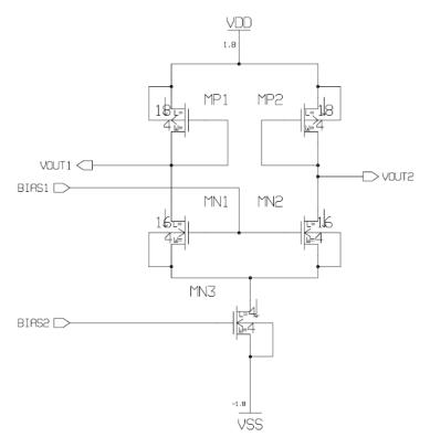
**Figure 4.2** The equivalent circuit of the SD-MAGFET. Circuit of the pMOS active load and the current sink is shown in this figure as well. The SD-MAGET is split into two nMOSs.
