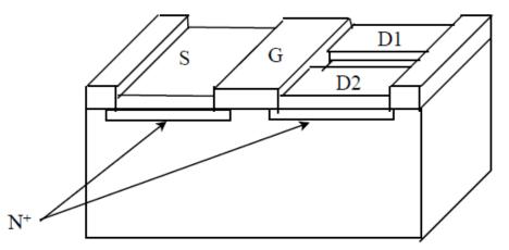
Figure 2.4 The three-dimensional view of the SD-MAGFET adapted from [5].
