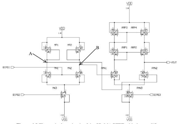
Figure 4.8 The equivalent circuit of the SD-MAGFET with the amplifier.
