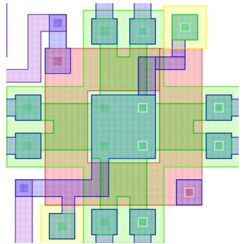
Figure 3.3 The entire layout design for the vertical magnetic field detection
