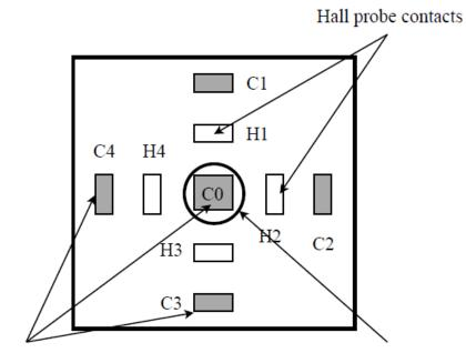
Power contacts P<sup>+</sup> Protective ring Figure 2.6 The square-shaped two-dimensional MFS adapted from [6].
