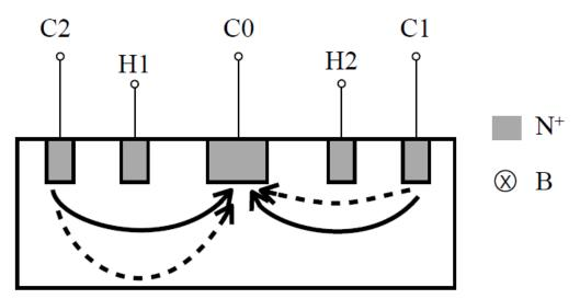
**Figure 2.5** The vertical Hall Plate has three Power contacts and two Hall probe contacts. C1 and C2 are connected with VDD, and C0 is connected with GND. Current will flow from C1 and C2 to C0. H1 and H2 are used to detect the variation of current caused by the magnetic field.
