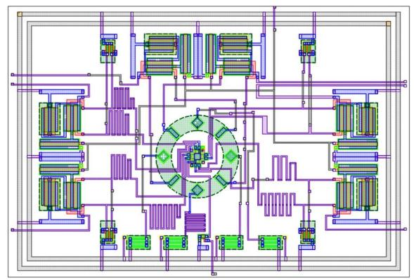
Figure 3.8 The entire layout of the three-dimensional MFS.
