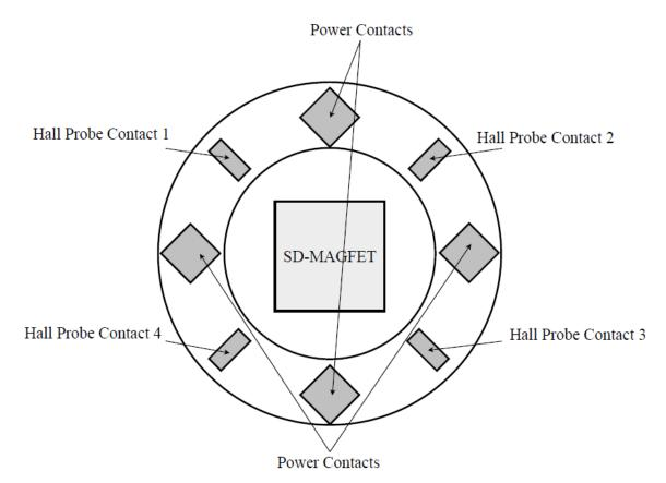
**Figure 3.6** The entire pattern of the three-dimensional MFS is shown in this figure. The SD-MEGFET which has the independent power supply is located at the center of the device. The detail of the circular VHD located around the SD-MAGFET is also shown in this figure.
