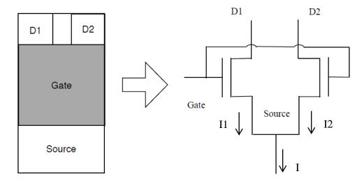
Figure 4.1 The equivalent circuit of the SD-MAGFET.
