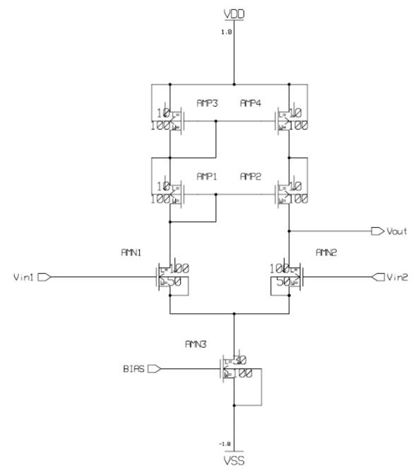
Figure 4.7 The equivalent circuit of the cascode amplifier.
