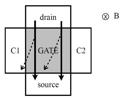
Figure 2.3 The top view of the horizontal MFS in the MOS structure adapted from [4].
