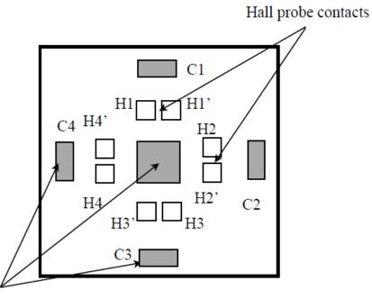
Power contacts Figure 2.9 The three-dimensional MFS with split Hall probe contacts adapted from [9].
