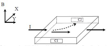
**Figure 2.2** A conventional Hall Plate which shows the current flow direction (solid line) and deflected current (dash line) by external magnetic field.
