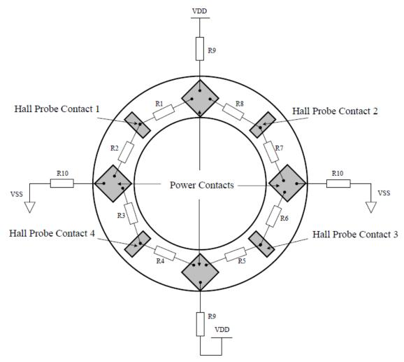
Figure 4.4 The conversion of the VHD in the form of resistor.
