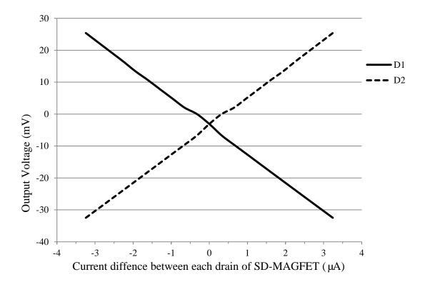
Figure 4.3 The output voltage swing of the SD-MAGFET.
