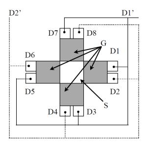
**Figure 5.1** Four right side drains and four left side drains are connected separately to increase the performance of the SD-MAGFET.
