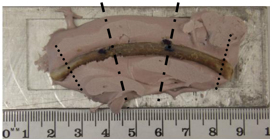
Figure 3.2 Depicted here is an 11 th beagle dog rib potted in Bondo ® and attached to an aluminum plate. This assembly was mounted on the slicer and three to four approximately cylindrical rib sections were obtained. Minor cuts made to the ends of ribs removed irregular bone geometry, depicted by dotted lines. Major cuts made to cut rib into cylindrical sections, depicted by dot hashed line.
