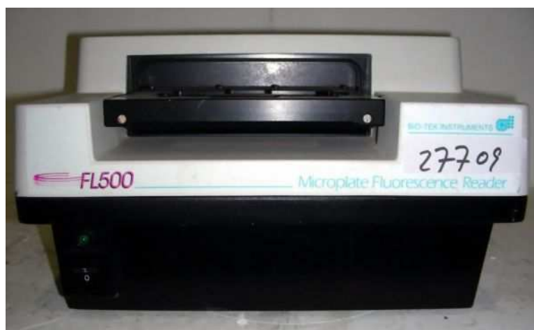
Figure 2.1 Microplate reader used for fluorescence spectrophotometry [3]. (Source: Manual for Bio-Tek Instruments FL500 Microplate reader, accessed on April,2011)
