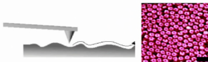
Figure 4.6 Scheme of contact mode imaging and an image of cholera oligomers [63].
