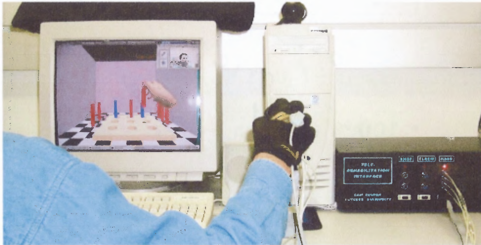
Figure 1.1 An example of Virtual Rehabilitation. In a simulated peg-board exercise, the user wears a haptic glove that translates his hand position and finger joint angles to an equivalent hand on screen. This can be repeated with precise starting positions for the pegs, and avoids loss or damage of equipment if physical pegs were used. As the glove does not offer tactile feedback, the user has to rely primarily on sight to determine exact positions.
