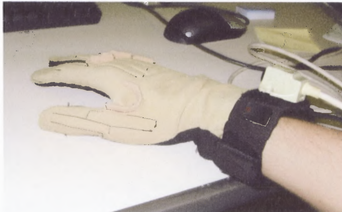
Figure 2.2 The CyberGlove® when worn on the right hand. The position sensor is attached to the top of the wrist using a Velcro pad. Because this is the only location it is attached to, it becomes inconvenient for the user, as it hangs below the attachment site and risks becoming entangled.
