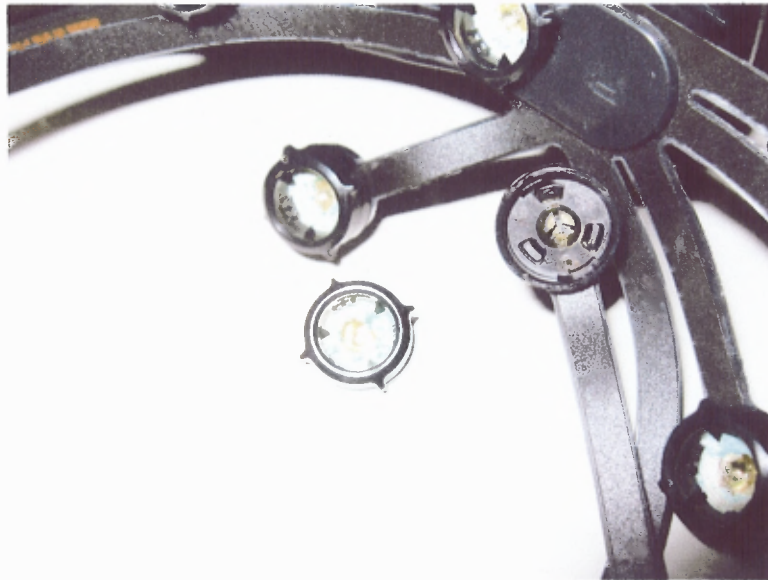
Figure 3.9 An electrode removed from its mounting is shown here, and the accumulation of electrolytic coating is also visible. The electrode itself is removed by twisting the electrode clockwise, allowing to substitute individual pads, though there are currently no replacements listed in the Emotiv online store.
