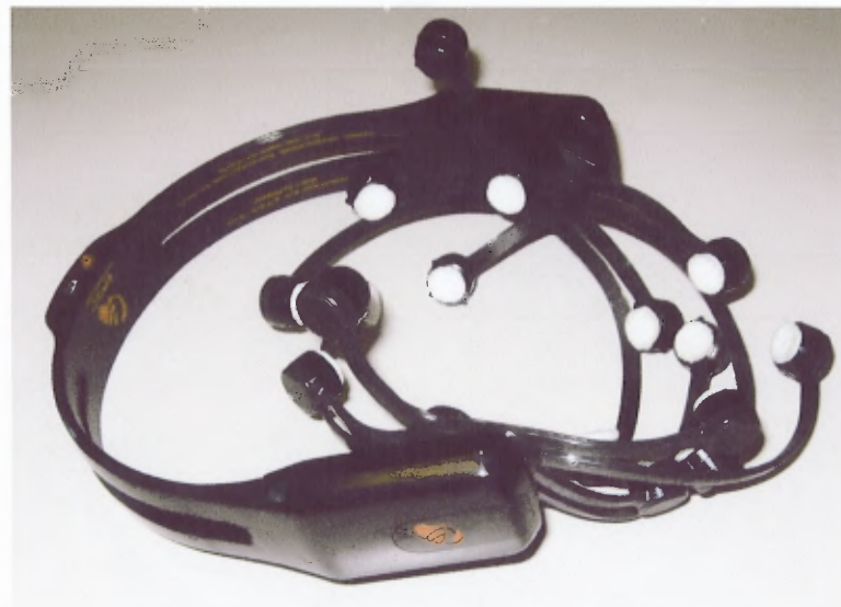
Figure 3.2 The Emotiv EPOC seen from the side, with the front facing to the right. The black pads are nonconductive Reference Electrodes, which are placed just behind the user's ears and are used to position the headset consistently.
