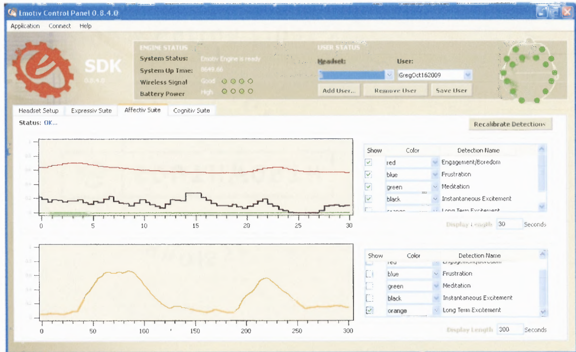
Figure 3.11 The Affectiv TM Suite is shown here. The display durations for the graphs are shown, as well as which emotional state is being measured on a relative scale from 0 to 1. Source: Taken at NJIT BME Motor Control and Rehabilitation Lab.
