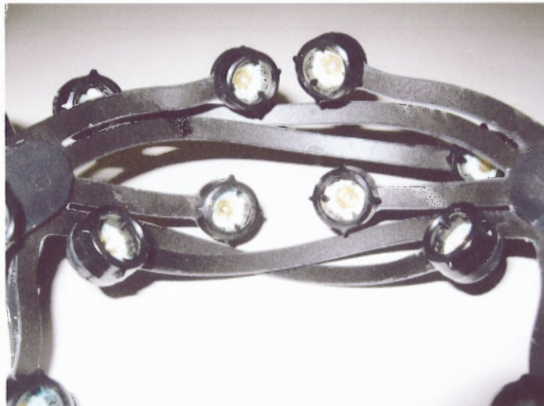
Figure 3.8 The EPOC™ electrodes are shown here without the pads. The green coating on the surface is not corrosion, but an electrolytic coating painted onto the gold contact plate that can migrate due to saline application.
