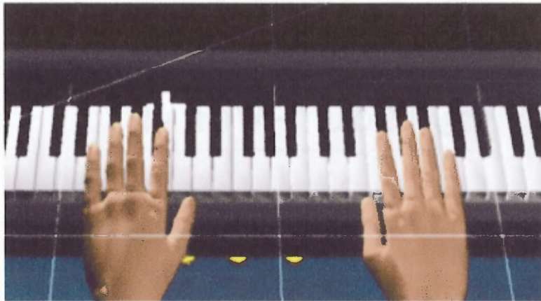
Figure 2.6 An image of the virtual hands in the Piano Training. In this experiment, both subjects had only one hand visible. The virtual hand maintains its orientation regardless of the orientation of the CyberGlove®, and can only move in the horizontal plane. The fingering and the corresponding key in each trial is highlighted in blue on the virtual hand.
