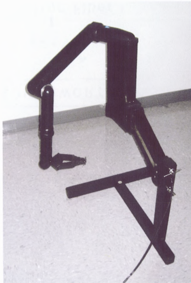
Figure 4.3 The iARM in a more stable position. This position can be maintained for longer periods of time than the previous one due to the reduced strain put on the joint motors, which is essential for repetitive testing. This position is also less likely to cause internal software errors, which require resetting of both hardware and software to resolve.
