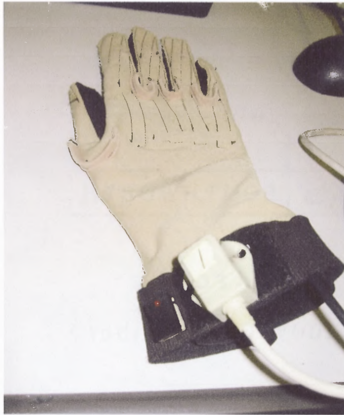
Figure 2.1 The CyberGlove®, when unworn.
