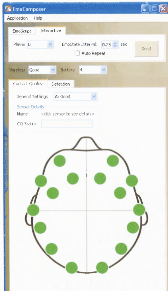
Figure 3.6 EmoComposer™ is shown here; the contact quality within Interactive Mode can be set when the ‘Contact Quality’ tab is clocked. Defaults include highest signal quality for all sensors, and noisy reference electrodes. Users can set each sensor individually.
