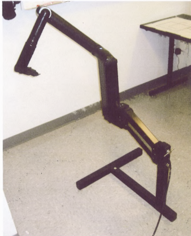
Figure 4.2 The iARM stops in this position once the ‘fold-out’ command is given. Source: Taken at NJIT BME Motor Control and Rehabilitation Lab.
