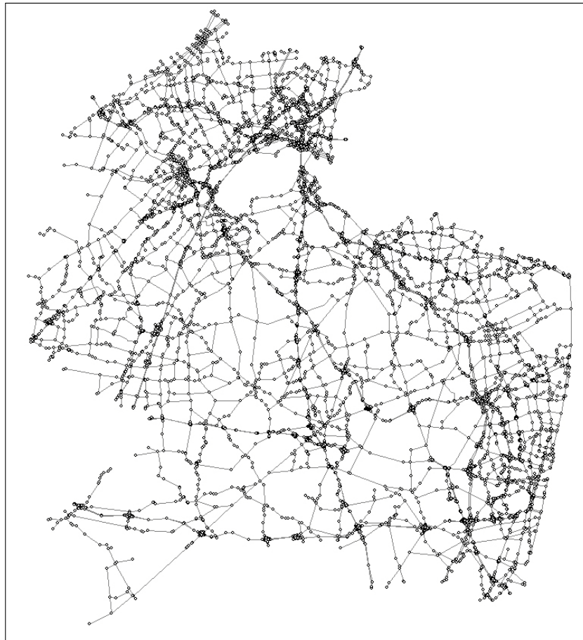
Figure 4.3 North Jersey regional trip-based TRANSIMS's model highway network.
